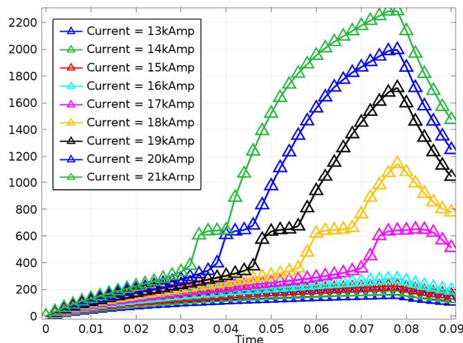
Fig 4 Timed temperature distribution of a point without pre heating
