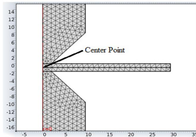
Fig 3 Mesh and center point at weld nugget
