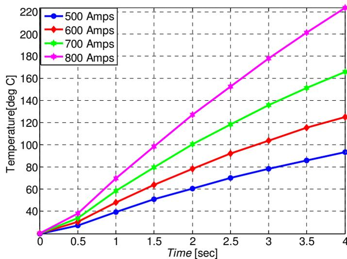
Fig 7 Heat distribution at center point with induction heating
