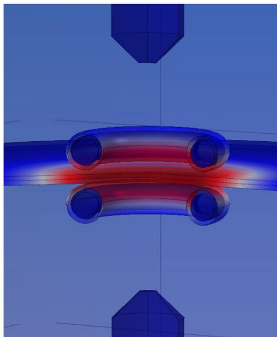
Fig 5 Induction heating for pre heating
