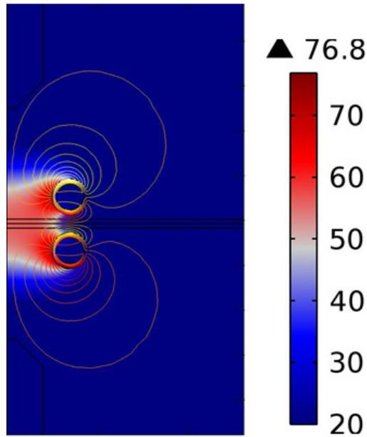
Fig 6 Magnetic flux density distribution [mTesla]
