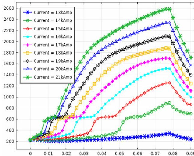
Fig 9 Timed temperature distribution of a point with pre heating 200°C
