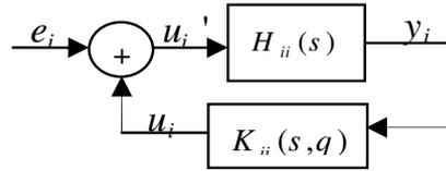
Fig. 5. Single input/Single output feedback system
