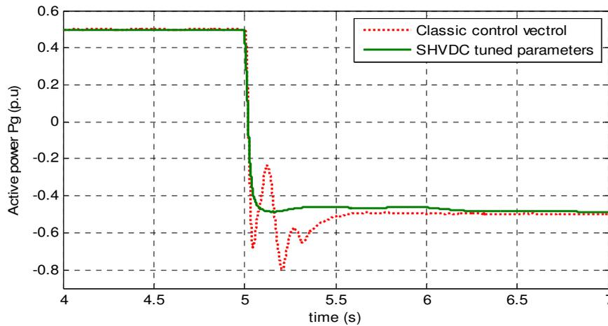
Fig.10. Response of  $P_g$  to -0.5 step in  $P_{g\_ref}$  (p.u)
