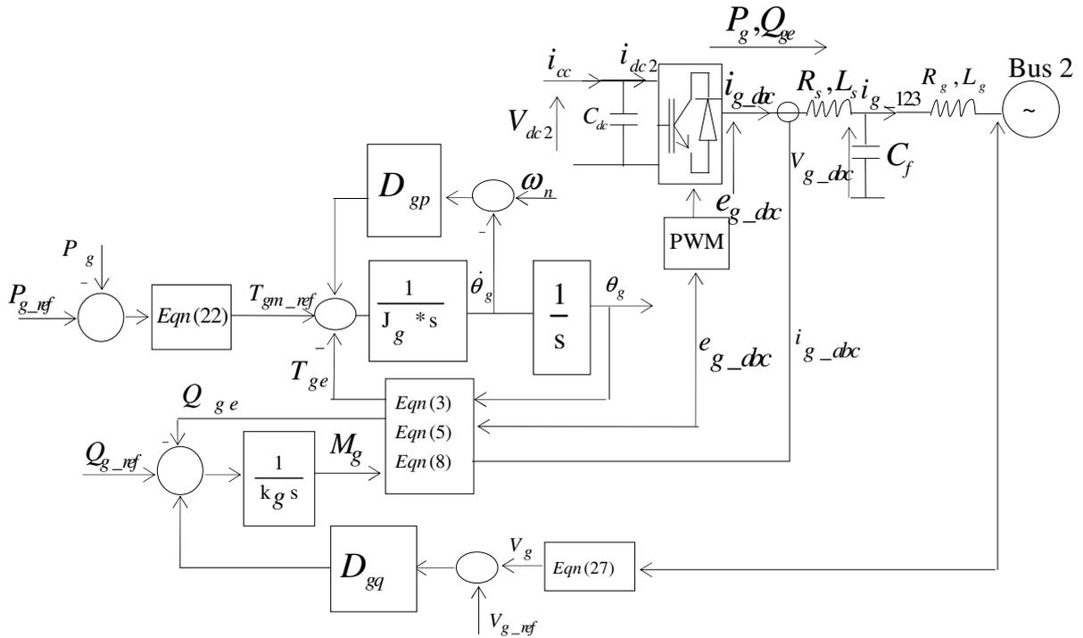
Fig. 3. Model of the synchronverter: power and electronic parts [17]
