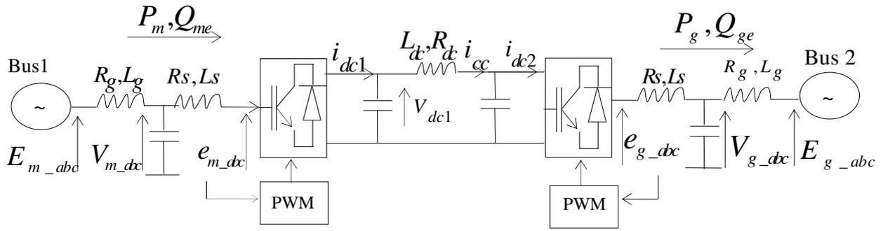
Fig. 2. Two terminal VSC-HVDC link
