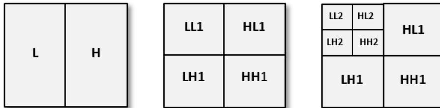
LL: low subbands for row and column filtering.      HH: high subbands for row and column filtering.
