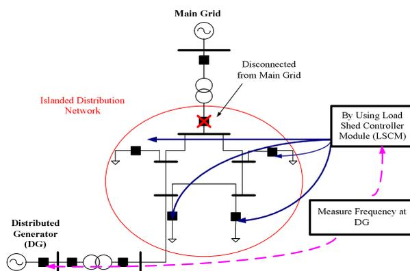
Fig.1. Principle operation of Load Shedding
