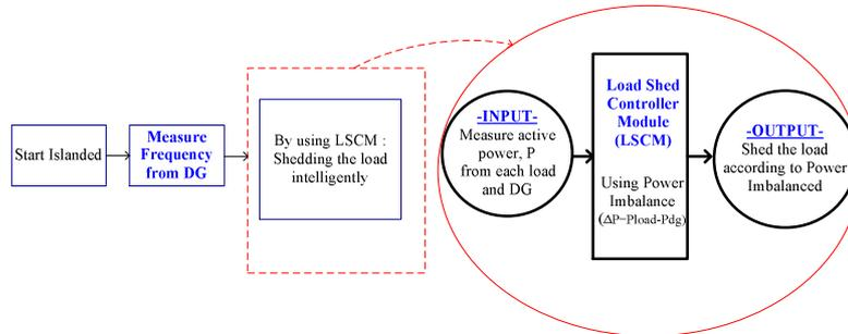
Fig.2. The development of Load Shedding Controller Module (LSCM)
