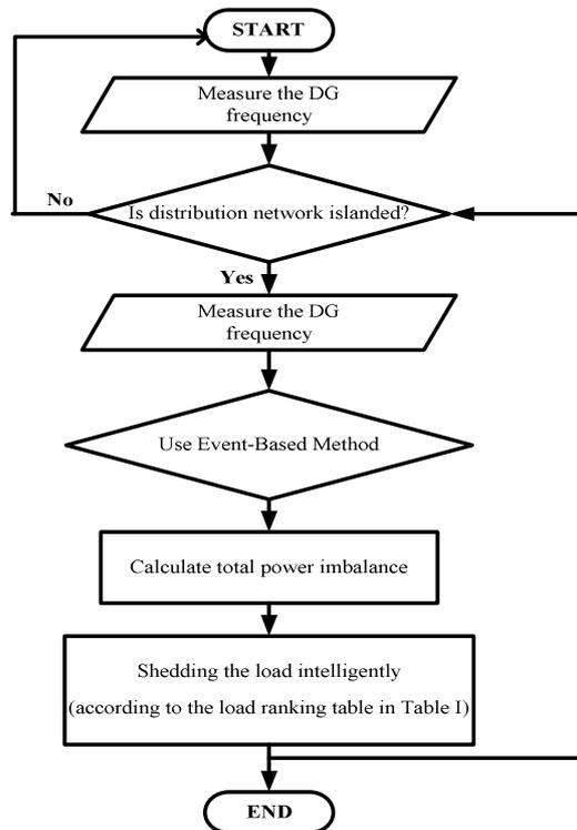
Fig.3. Principle operation of UFLS for event-based
