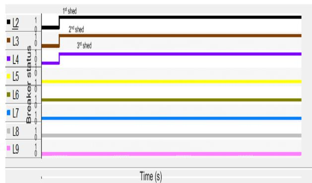
Fig.10. Breaker status of each load for peak load condition
