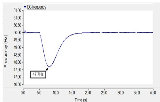
Fig.9. System frequency response with load shedding
