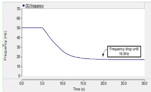
Fig.8. System frequency response without load shedding
