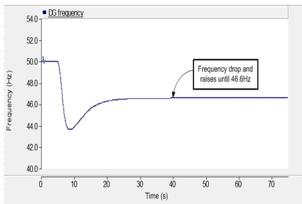
Fig.5. System frequency response without load shedding
