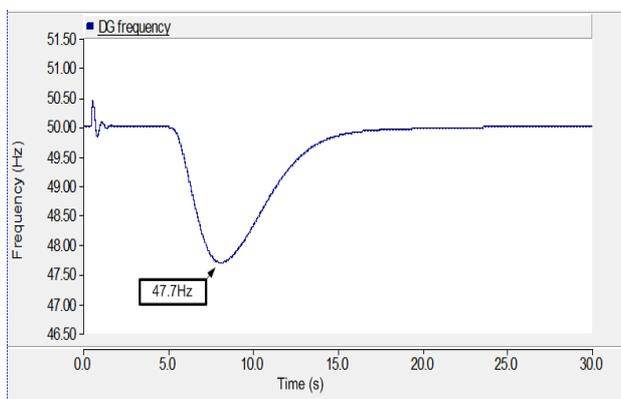
Fig.6. System frequency response with load shedding
