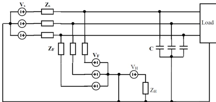
Fig. 7. Equivalent circuit of the system in Fig. 6 under sinusoidal steady state.
