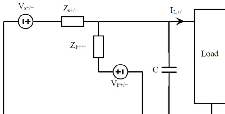
Fig. 8. Positive/negative sequence circuit for the circuit shown in Fig. 7.
