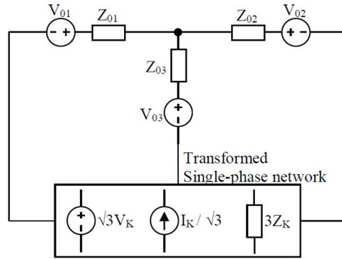
Fig. 5. Zero sequence circuit of Fig. 4 with the single-phase network reported through the ideal transformers.
