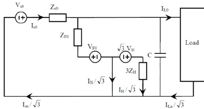
**Fig. 9.** Zero sequence circuit of the circuit in Fig. 7. The single-phase network and the related variables are represented according to the analytical results derived in Section 3.
