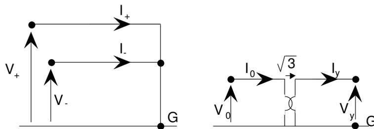
Fig. 2. Symmetrical-components equivalent circuits of a star connection: positive and negative sequence circuits on the left, and zero sequence circuit on the right.
