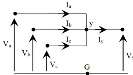
Fig. 1. Star connection between a three-phase and a single-phase network.
