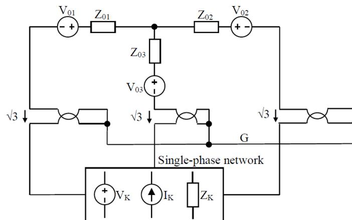
Fig. 4. Zero sequence circuit for the sample network shown in Fig. 3.
