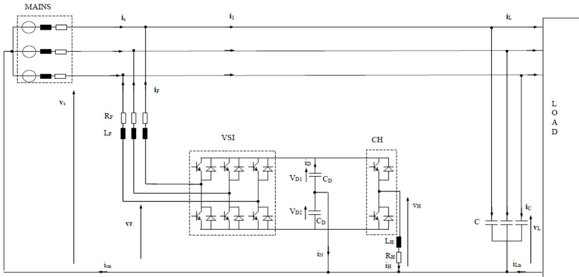
Fig. 6. Application example used to illustrate the theoretical results derived in Section 3. The system includes a three-phase voltage source inverter connected to a half-bridge inverter (i.e., a single-phase network).
