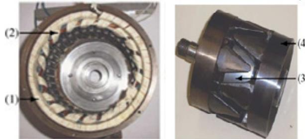
Figure 1: Built prototype of the SE2A. Legend: (a) Sator of the SE2A, (b) rotor of the SE2A, (1) half of the statorDC-excitation ring winding, (2) armature en winding, (3) non-magnetic core, (4) magnetic collector
