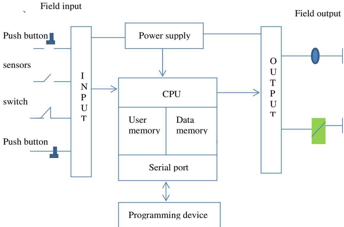
**Fig. 1:** Internal Block Diagram of PLC
