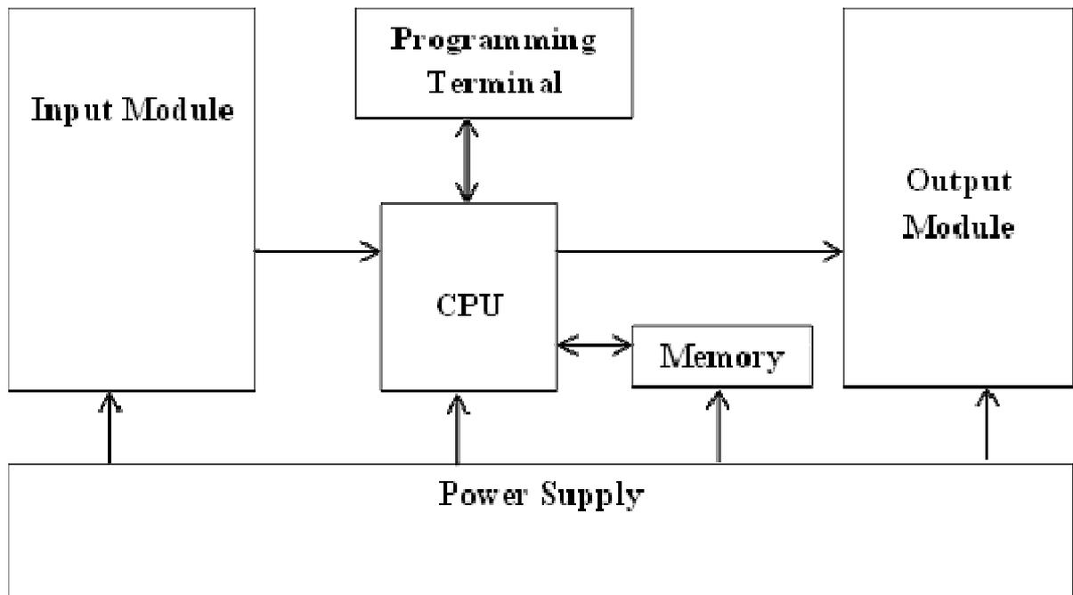
Fig.5: PLC Hardware Block Diagram
