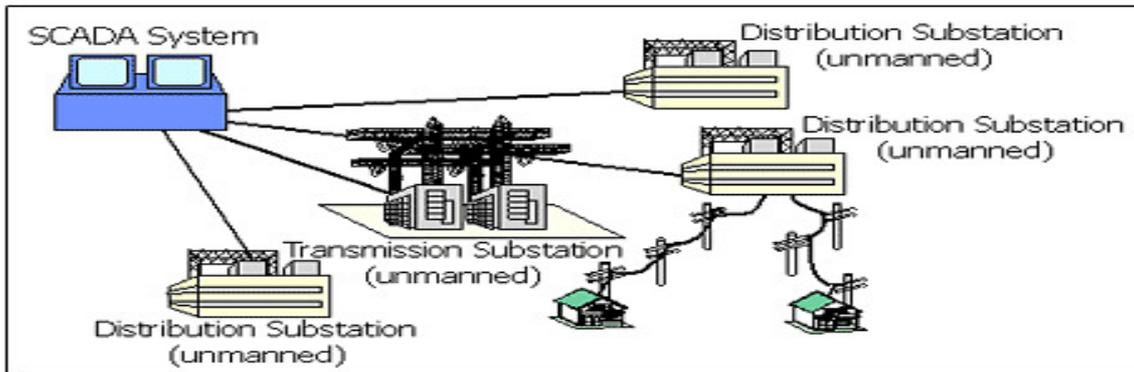
Fig. 2: Basic Structure of SCADA System
