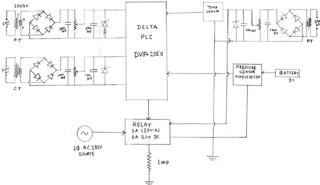
Fig.4: Circuit diagram of Automation of the Sub-Station
