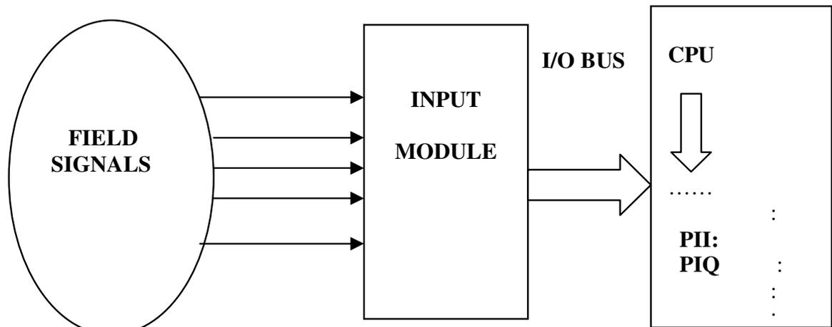
Fig.6: Working of PLC
