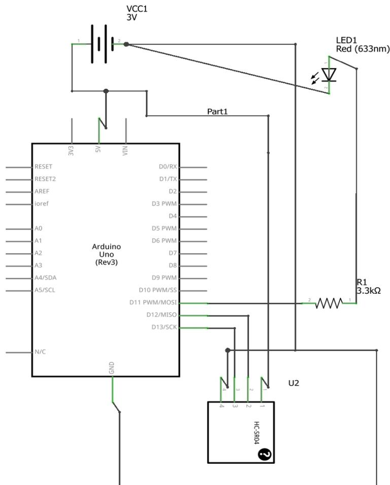
Fig. 5 LED connection functional scheme as the signaling lamp
