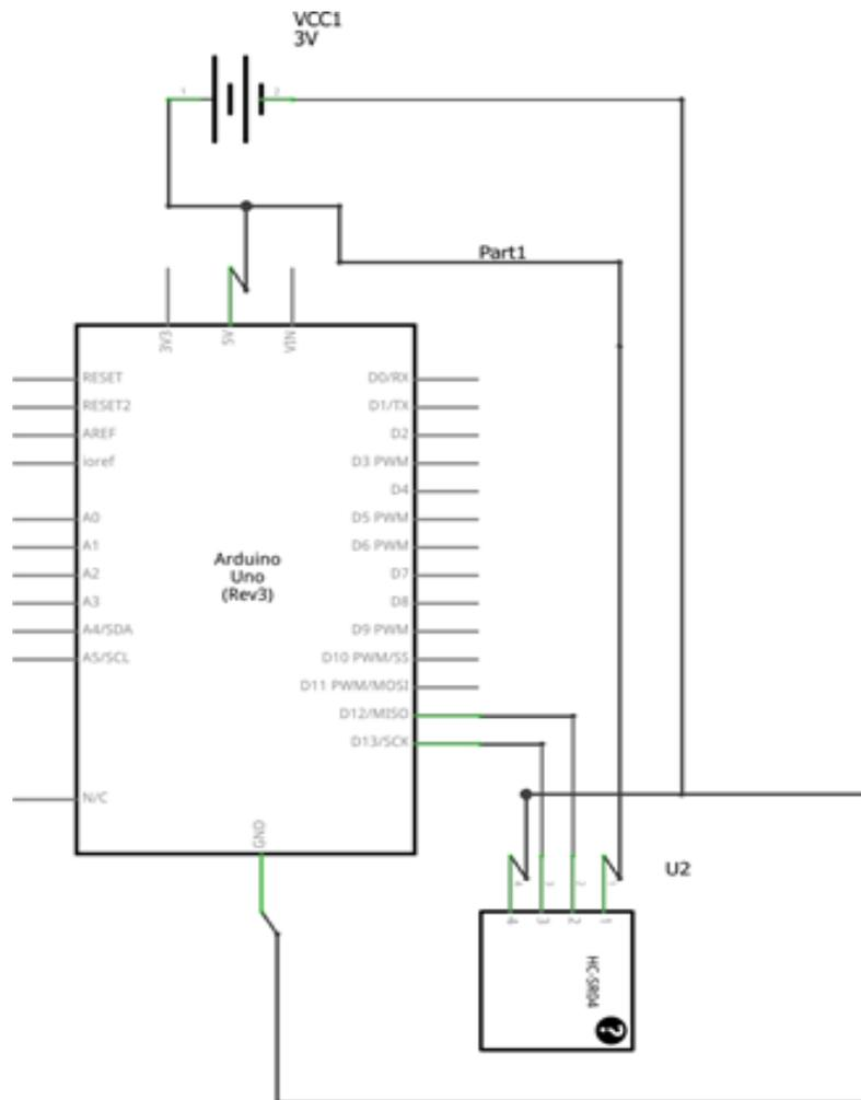
Fig. 3 Scheme of the distance sensor connection HC-SR04
