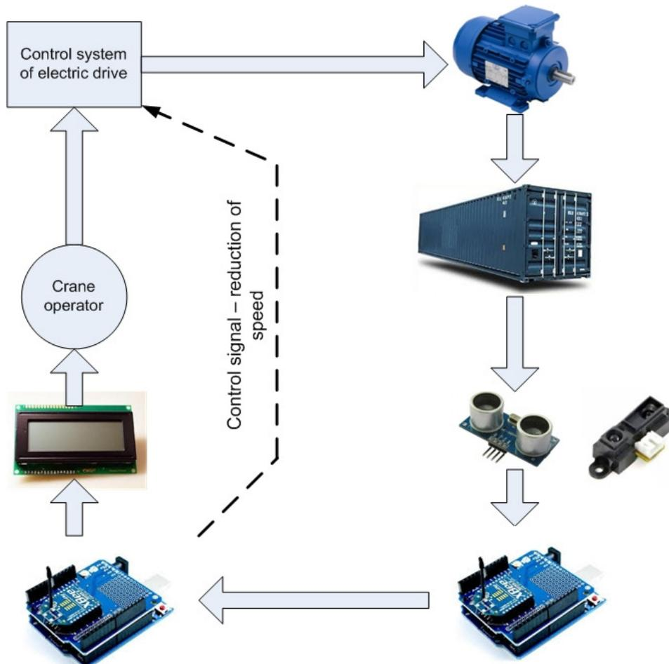
Fig. 1 Scheme of the experimental complex under development
