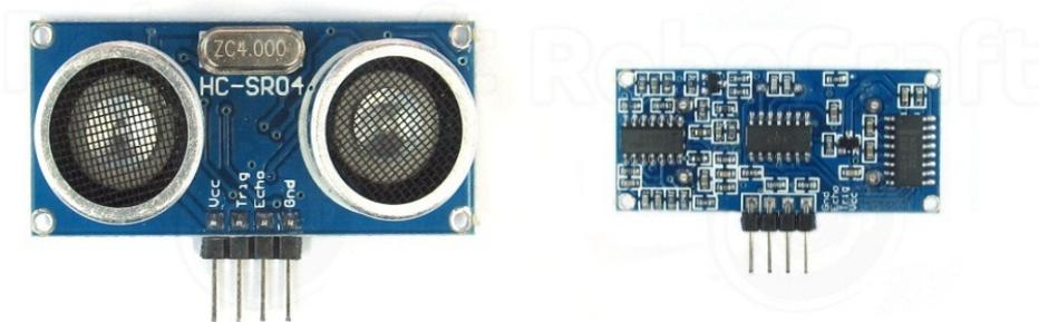
Fig. 2 Physical form of the ultrasonic sensor HC-SR04
