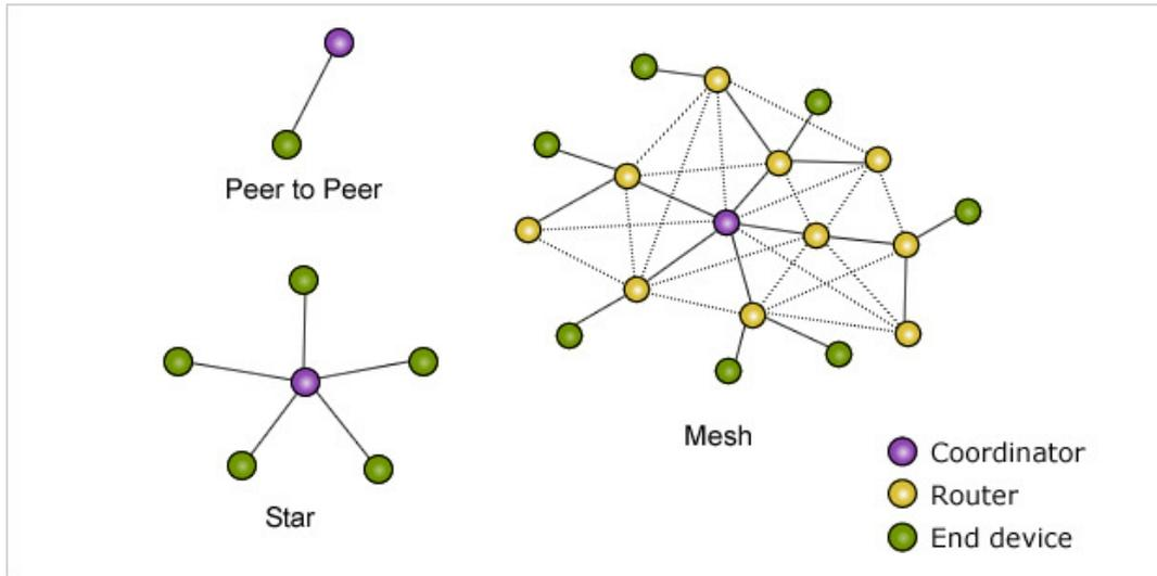
Fig. 4 Various ZigBee/802.15.4 network topologies
