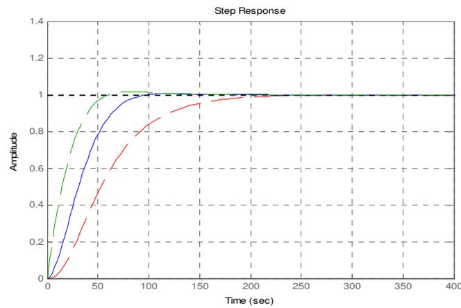
Figure 6. Step responses of the reference and tracking bound models.
