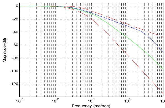
Figure 12. Upper and lower magnitude envelopes of closed loop system.
