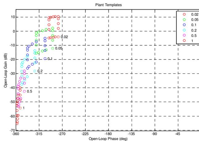
Figure 4. Ship model templates for six frequency values.
