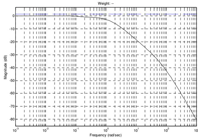
Figure 13. Robust stability verification for course changing autopilot.
