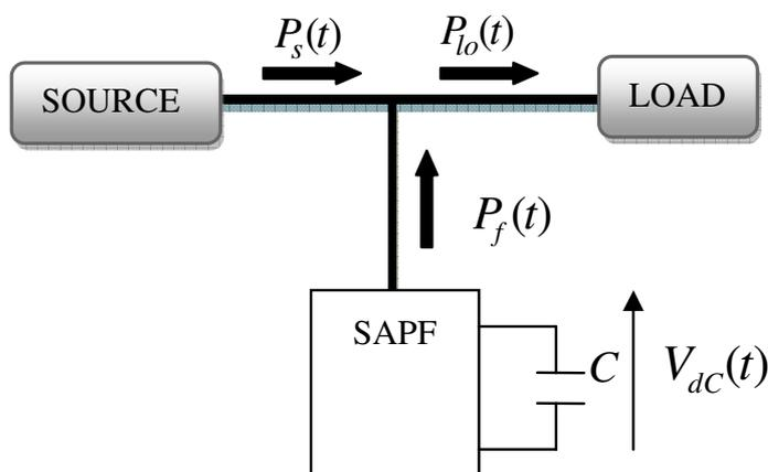
Fig. 4 power Exchange between network, load and filter
