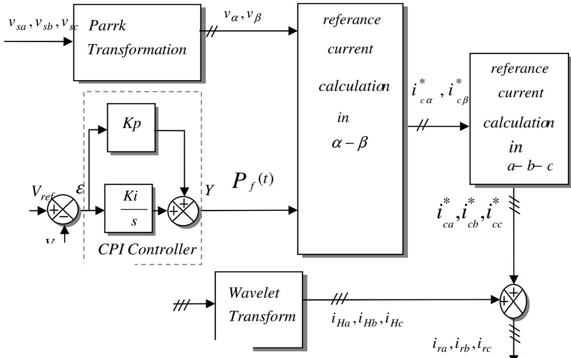
Fig. 6 Block diagram for the Wavelet transform method
