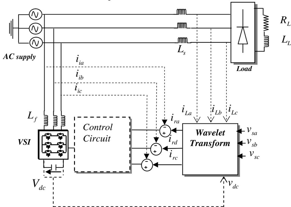
Fig. 1 Schematic diagram of shunt APF
