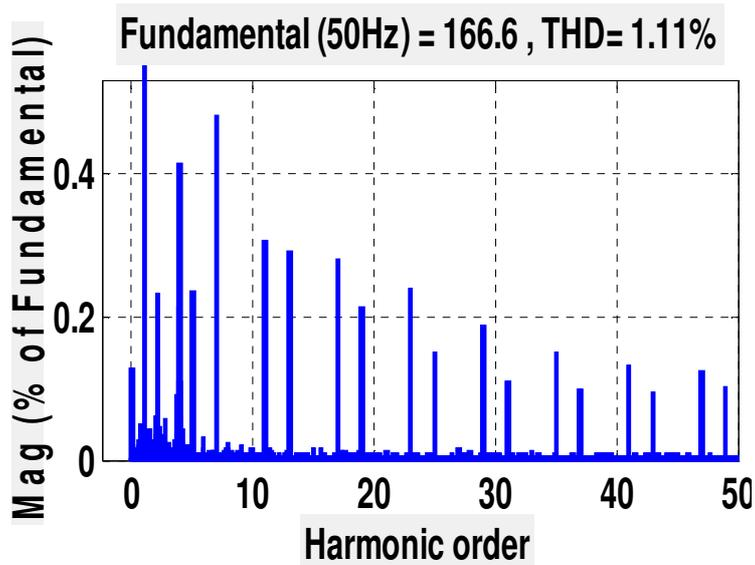
Fig. 12 Harmonic spectrum of supply current ( Phase -a-)
