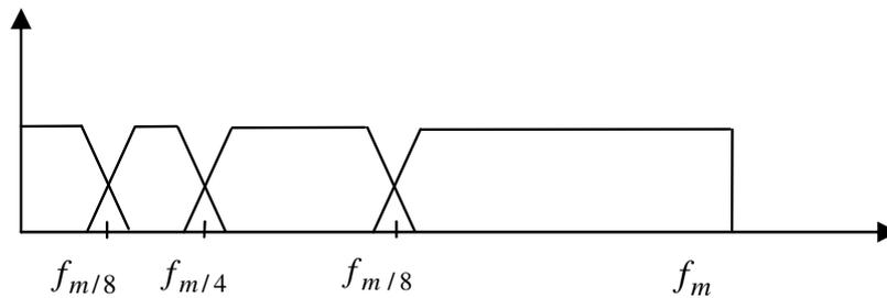
Fig. 3 Spectral characteristics for 3-level decomposition
