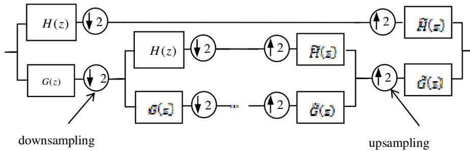
Fig. 2 Implementation of the filters bank for the Discret Wavelet Transform
