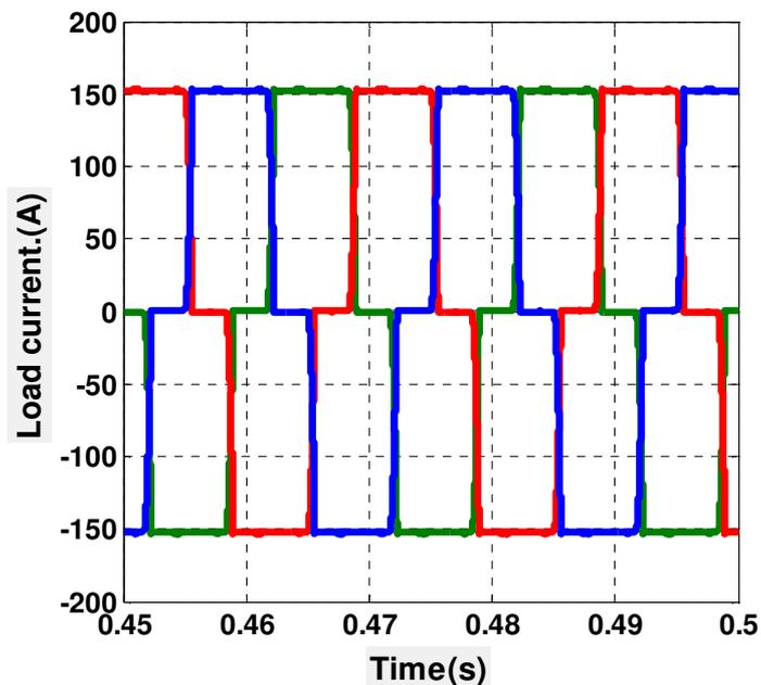
Fig. 8 Simulated of load current
