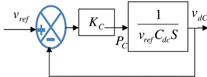
Fig. 5 Control loop of the DC voltage
