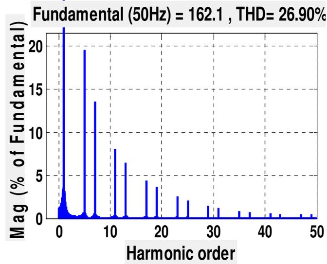
Fig. 9 Harmonic spectrum of load current (Phase -a-)
