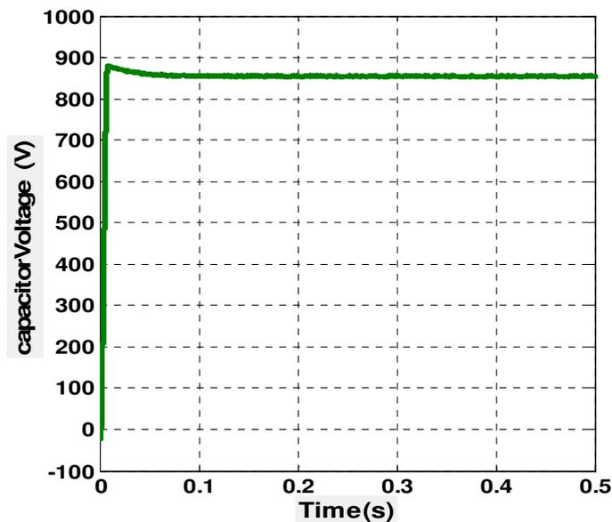
Fig. 13 DC link voltage regulation
