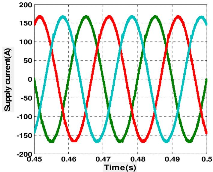
Fig. 11: Simulated of supply current waveforms
