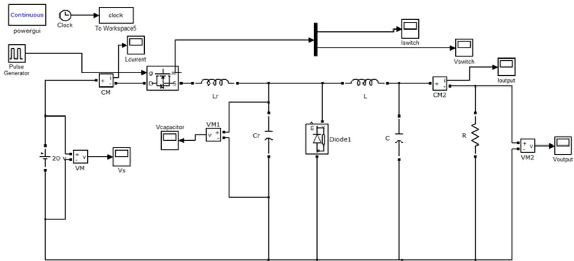
Fig.3.2 Simulink model of ZCS based Buck converter
