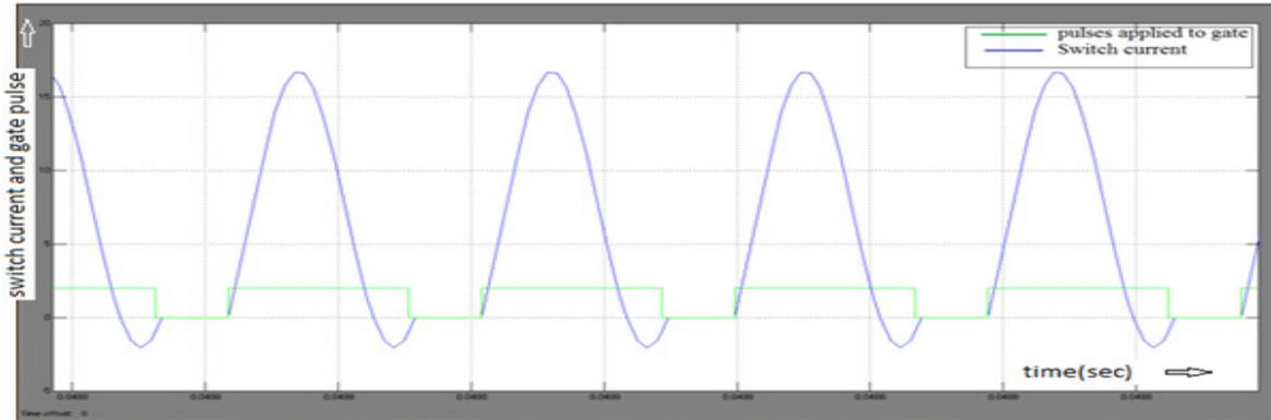
Fig.3.8 switch (MOSFET) current and pulse of ZCS based buck converter
