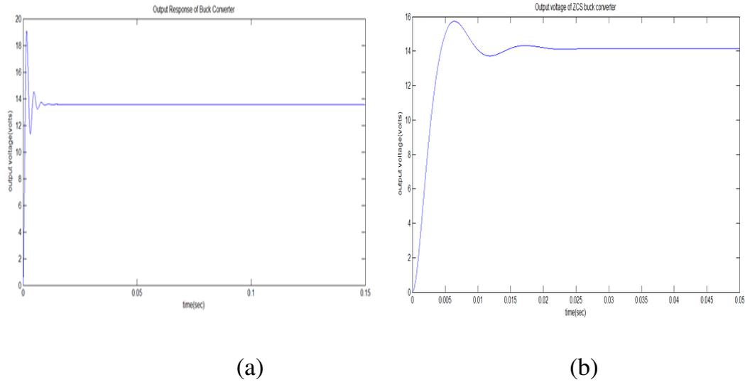
Fig.3.4 Average output voltage responses of buck and ZCS based Buck converters
