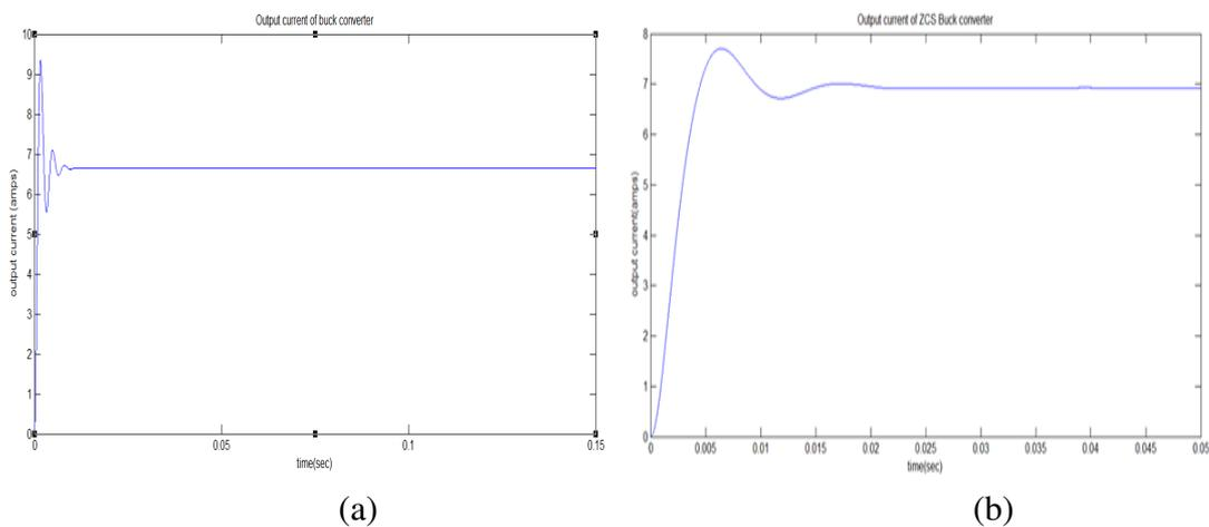
Fig.3.5 Average output current responses of buck and ZCS based Buck converters
