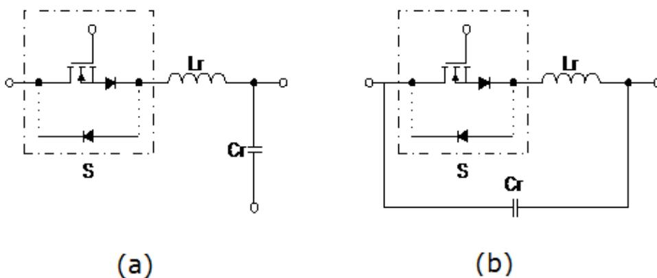
Fig.2.5 ZC Resonant switch.
