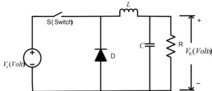
Fig.2.1 Buck Converter
