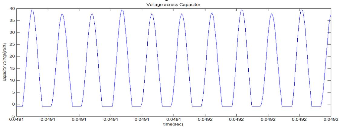
Fig.3.9 Voltage response of the resonant capacitor in ZCS based buck converter
