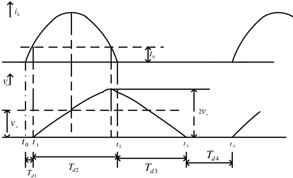
Fig.2.7 Model waveforms of ZCS converter
