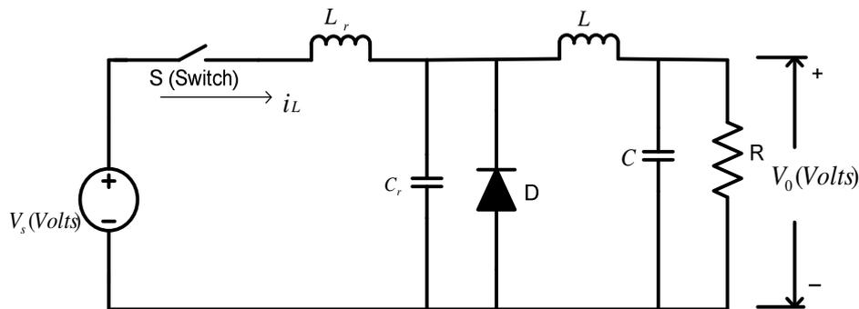
Fig.2.6 ZCS Based Buck converter
