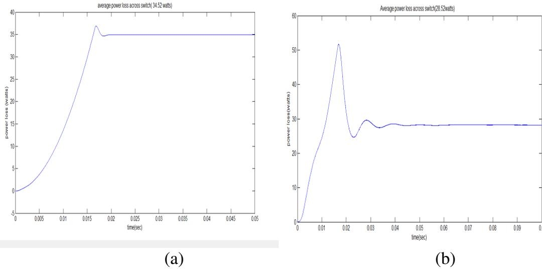
Fig.3.6 Average power loss across the switch (MOSFET) of buck and ZCS based Buck converters
