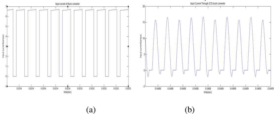
Fig.3.3 Supply Current of buck and ZCS based Buck converters.
