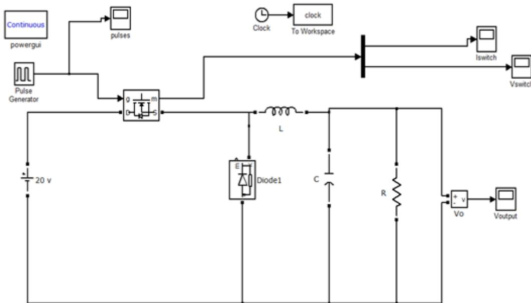
Fig.3.1 Simulink model of Buck converter
