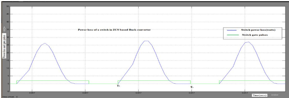
Fig.3.7 Power loss across the switch (MOSFET) of ZCS based buck converter
