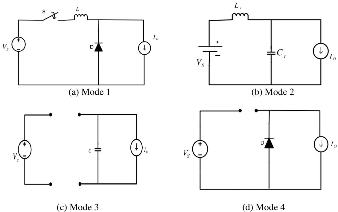
Fig.2.8 Modes of operation of ZCS converter
