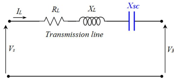
Figure 1. Single transmission line with SC.
