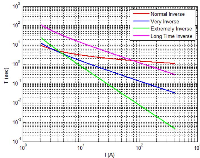
Figure 4. Time-current of IDMT overcurrent relaying characteristics.
