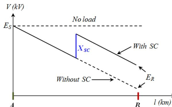
Figure 2. Voltage profile on transmission line with SC.
