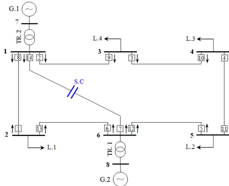
Figure 7. Single line diagram of the 8-bus network with SC.
