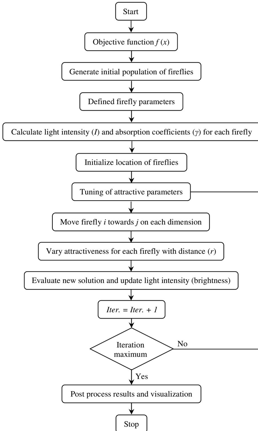
Figure 6. Schematic Flowchart of the FA.
