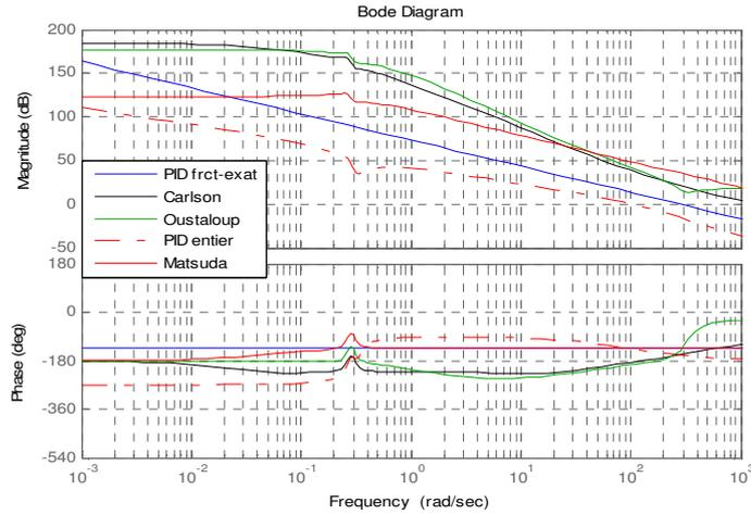
Figure 7 Bode's diagrams of the current  $i_d$  (state  $x_1$ ) controlled by classical PID and FOPID with various approximations
