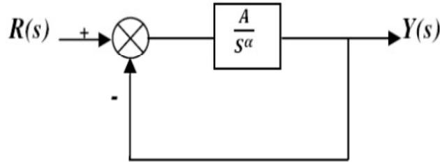
Figure 1 Diagram of Bode's ideal loop (BIL)
