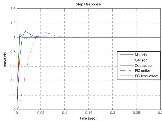
Figure 8 Step responses of the current  $i_q$  (the state  $x_8$ ) controlled by classical PID and FOPID with various approximations
