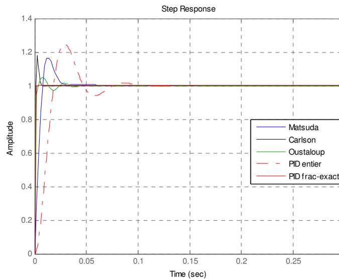
Figure 6 Step responses of the current  $i_d$ (state  $x_1$ ) controlled by classical PID and FOPID with various approximations
