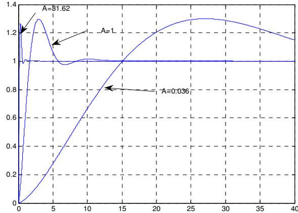
Figure 2 The step responses of the BIL for  $\alpha = 1.5$  and various values of A
