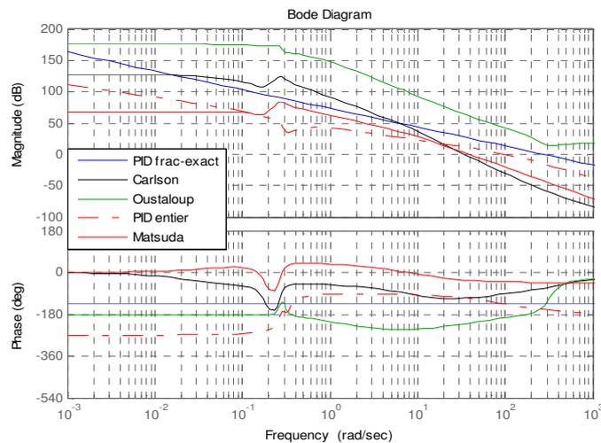
Figure 9 Bode's diagrams of the current  $i_q$  (state  $x_8$ ) controlled by classical PID and FOPID with various approximations
