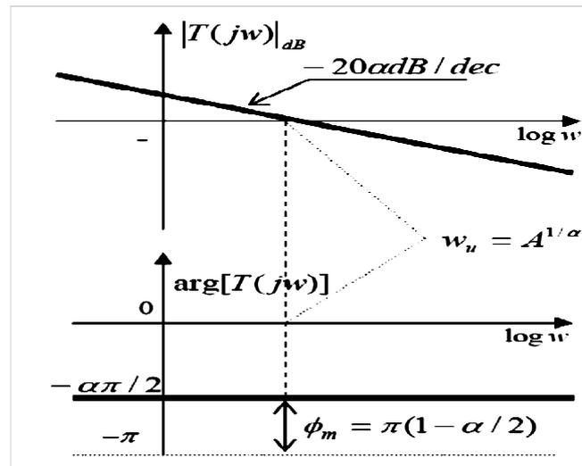
Figure 3 Bode's diagram in open-loop of BIL
