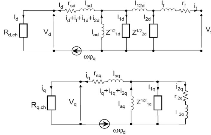
Figure 5 Non integer order d and q-axis equivalent circuits of a synchronous machine
