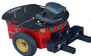
Figure 1. The robot Pioneer II.
