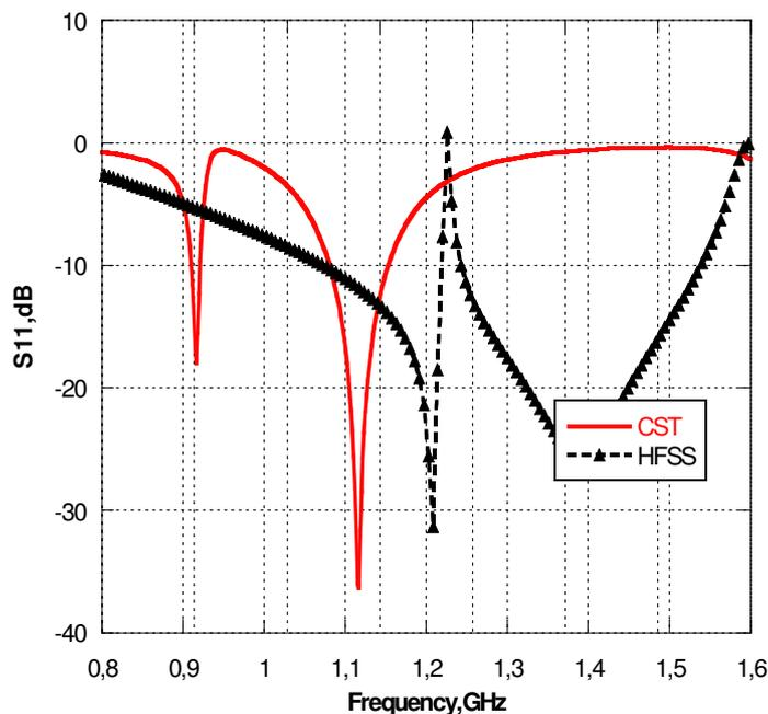
Figure 9 S11 simulation results comparison between HFSS and CST.
