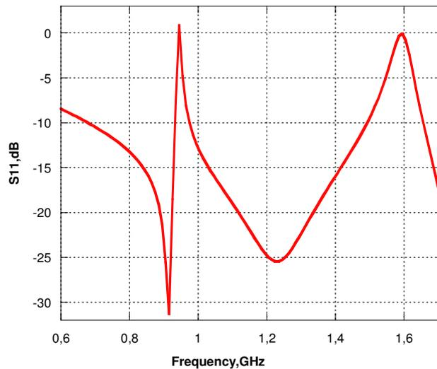
Figure 6 HFSS antenna simulated return loss.
