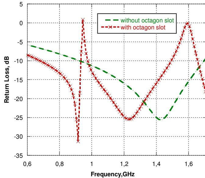
Figure 4 The ground octagon slot effect on the return loss.
