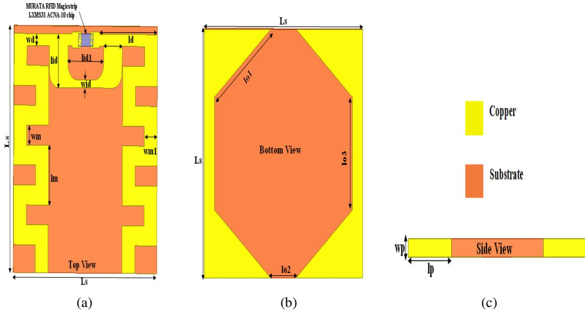
Figure 1 The proposed antenna structure (a) Top view (b) Bottom view (c) Side view.
