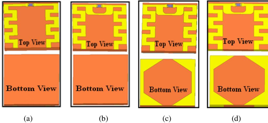
Figure 2 The proposed antenna design procedure (a) Antenna I (b) Antenna II (c) Antenna III (d) Proposed Antenna.
