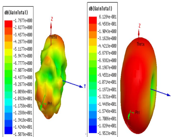
Figure 5 The ground octagon slot effect on the maximum gain: (a) with full ground plane (b) with slotted ground plane.
