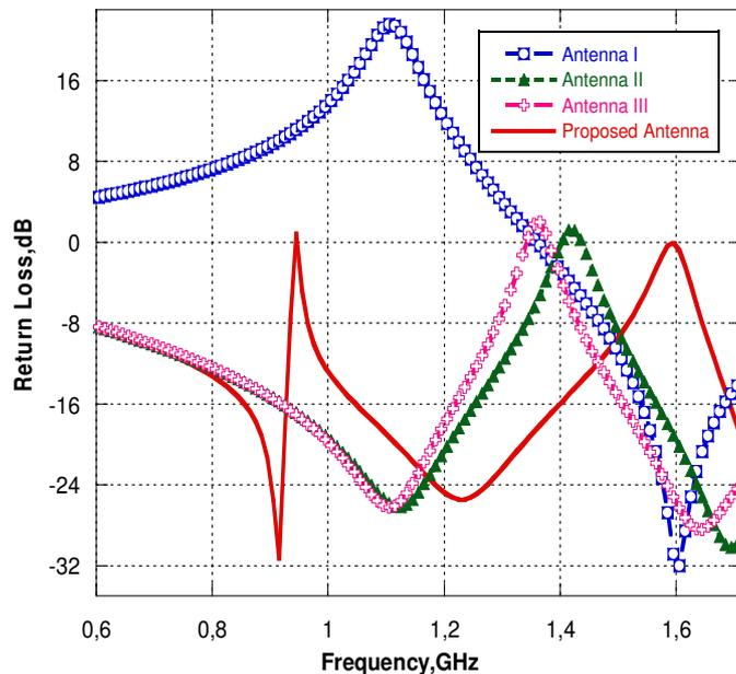
Figure 3 Compared return loss of the designs antenna.
