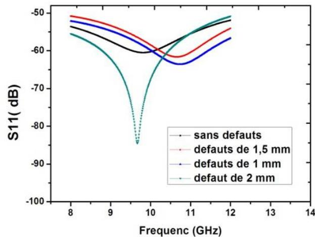
Figure 7. Variation of reflection coefficient (S11) depending on the depth of the defects
