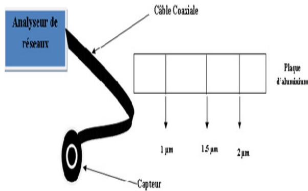
Figure 1. Measurement system and detection of defects.
