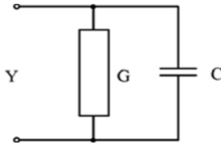
Figure 2. Equivalent circuit of a probe. [14]
