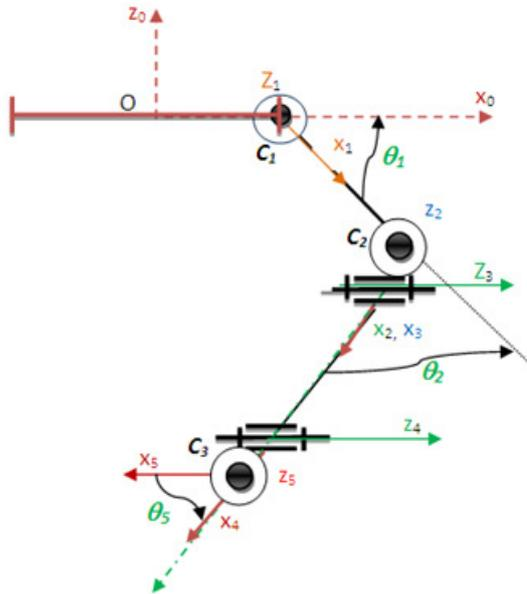
Figure 6 Parameters of arm3 of the Par 4
