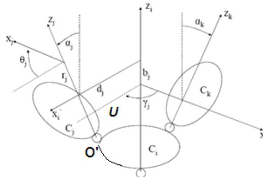
Figure 2 The MDH parameters for tree structure robot.
