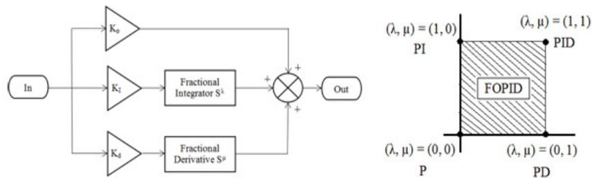
Figure 2. Generalized Fractional Order PID controller
