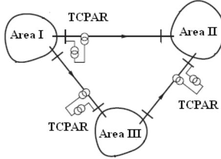
Figure 3. Test system with TCPAR in tie-lines
