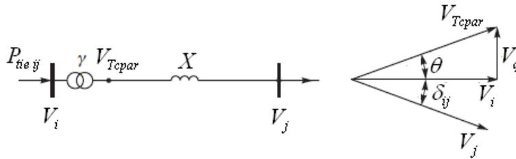
Figure 4. Single line diagram of TCPAR and phasor diagram
