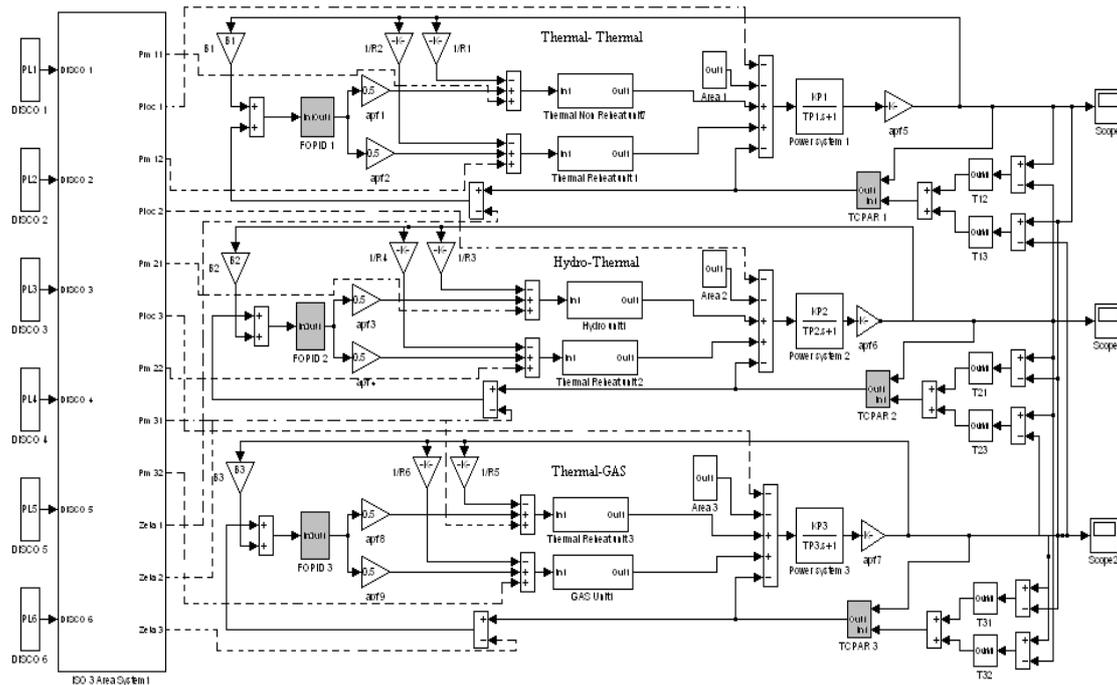
Figure 1. Three area composite deregulated power system
