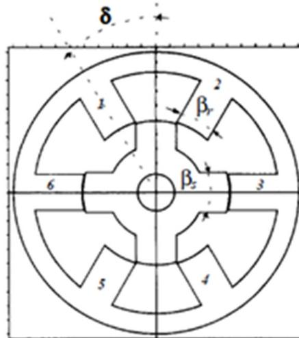
Figure 2 The angle  $\delta$  corresponding to displacement of a phase in relation to another
