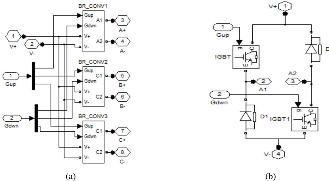
Figure 5 H-bridge asymmetric converter: (a) Power converter detail, (b) Phase detail
