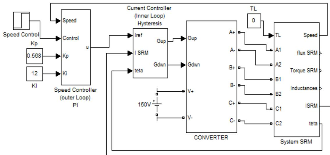
Figure 3 Matlab/Simulink diagram of SRM linear model
