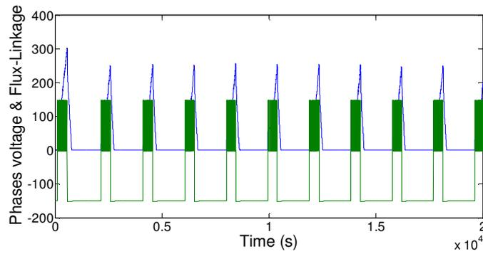
Figure 10 Phase Voltage and Flux-Linkage
