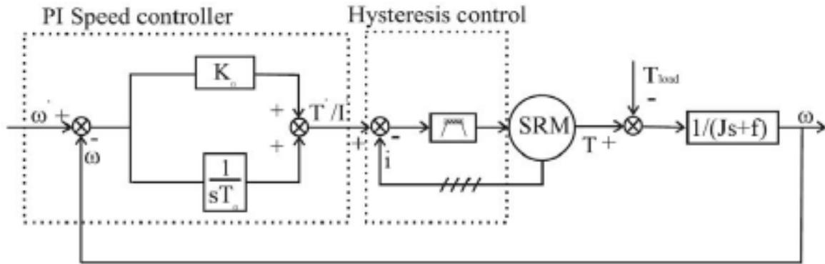
Figure 6 Closed-loop speed and current control block diagram of a SRM [11]
