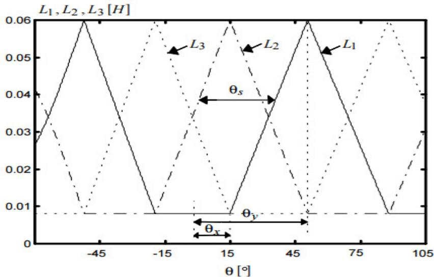
Figure 1 SRM linear model. Inductance profile of each phase
