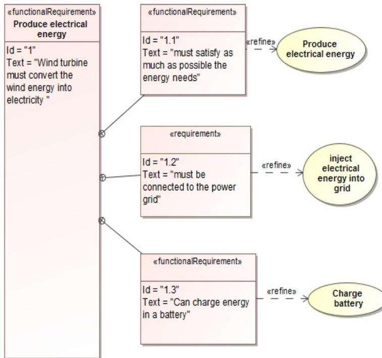
Fig. 3. Functional requirements diagram
