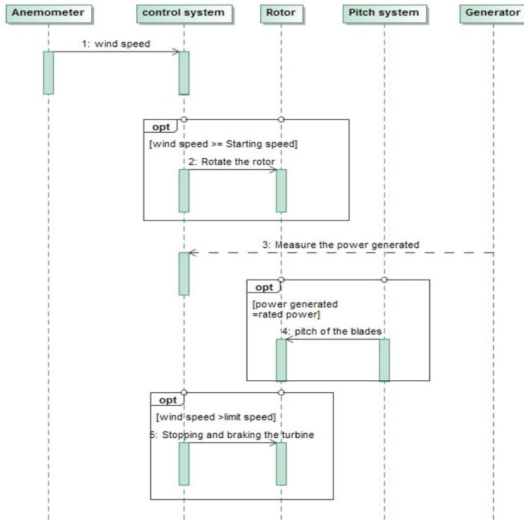
Fig. 5. Performance requirements diagram
