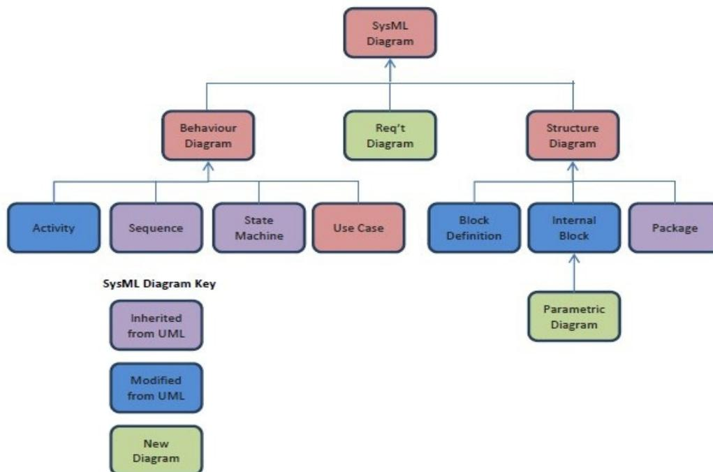
Fig. 1. SysML 1.0 diagram architecture.
