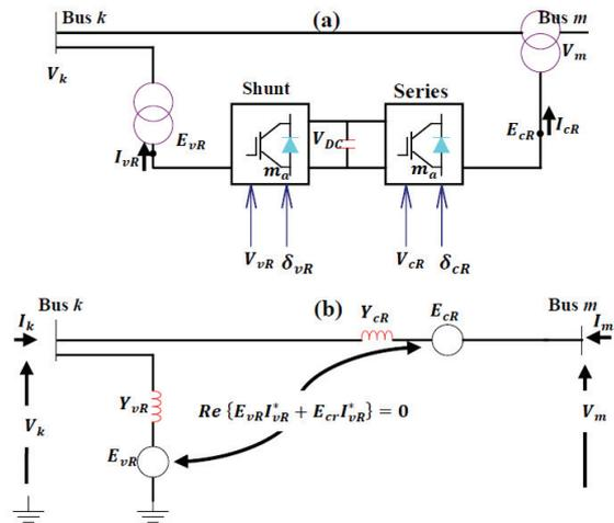
Fig.1. The UPFC equivalent circuit
