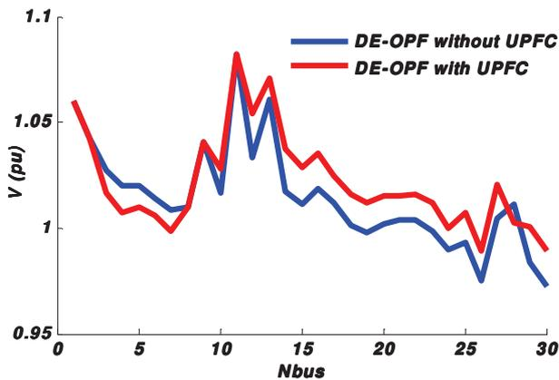
Fig.5. Voltage profile of all buses for IEEE 30-Bus with & without UPFC
