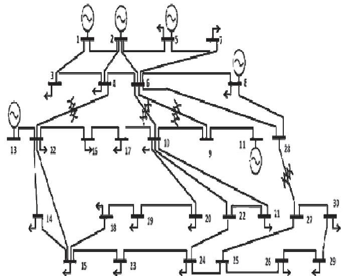
Fig. 3. Topology of the IEEE 30-Bus electrical network
