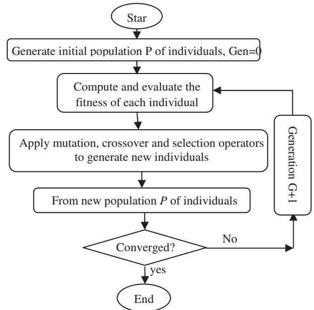
Fig.2 optimal power flow using DE
