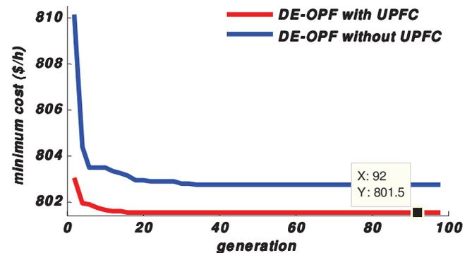
Fig. 4. The convergence profile of DE-OPF with/without UPFC for IEEE 30-bus system
