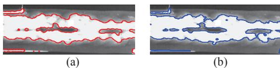
Fig.5. Detection of defects in weld radiographic image by proposed method. (a) Initial contour; (b) Final segmentation after 150 iterations.
