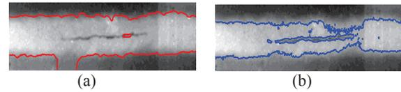
Fig.7. Detection of defects in weld radiographic image by proposed method. (a) Initial contour; (b) Final segmentation after 150 iterations.
