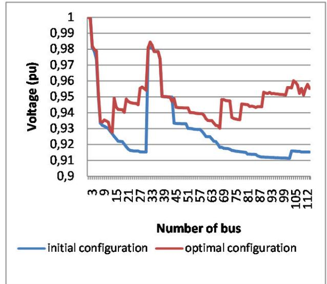
Fig. 7. Level voltage of each bus of the distribution real network 112-bus before and after reconfiguration
