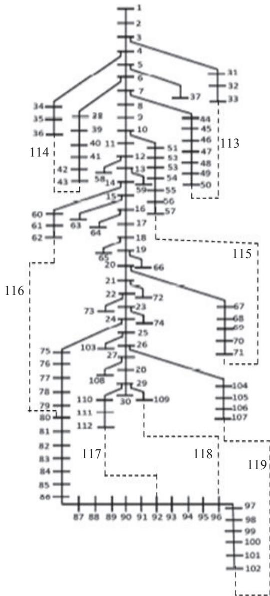
Fig. 6. Real distribution network 112-bus with normally open switches (tie-switches).
