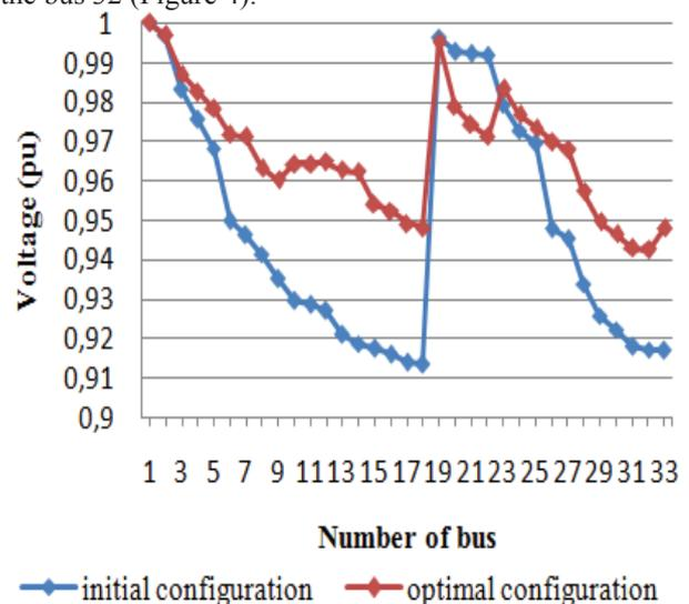
Fig. 4. Level voltage of each bus of the distribution IEEE33-bus before and after reconfiguration
