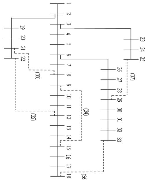
Fig. 3. IEEE33-bus with normally open switches (tie-switches)
