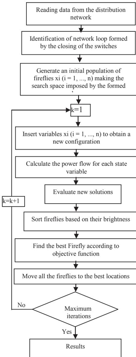
Fig. 2. Flowchart of the determination of the optimal topology of the distribution network
