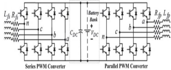
Fig. 5. Two three-phase four-leg converters based Grid Emulator [10]
