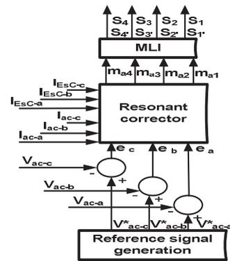
Fig. 9. EUT side converter control strategy
