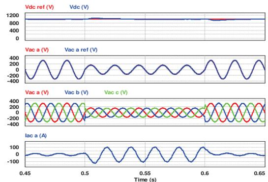
Fig. 11. Simulation results of the proposed grid emulator connected to the EUT (photovoltaic inverter) and three-phase RL load in presence of voltage sag conditions
