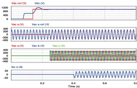
Fig. 10. Simulation results of the proposed grid emulator connected to the EUT (photovoltaic inverter) and three phase RL load in ideal grid operating conditions
