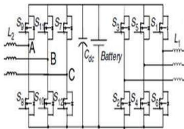
Fig. 4. Two conventional three-phase three-leg converters based Grid Emulator [9]
