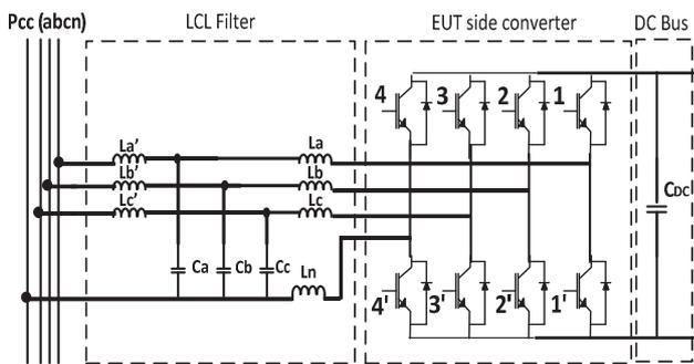
Fig. 7. The designed AC and DC Grid Emulator filters
