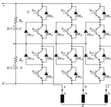
Fig. 2. Three-Level Neutral Point Clamped Voltage Source Converter (3L-NPC-VSC) based Grid Emulator [7]
