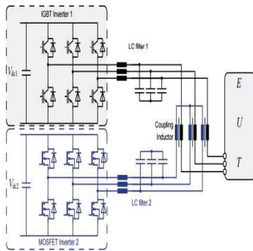
Fig. 3. Voltage Source Inverter Cumulation based Grid Emulator [8]
