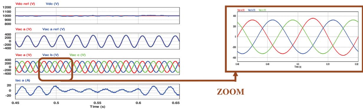
Fig. 12. Simulation results of the proposed grid emulator connected to the EUT (photovoltaic converter) and three phase RL load under unbalance fault conditions
