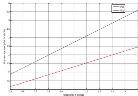
Fig.7. Upstream power variation in 33-bus system with uncertainty in the variation of loads without installing DG.
