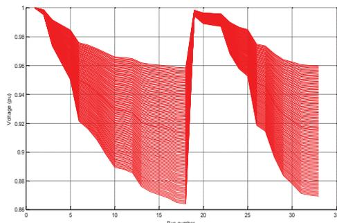
Fig.5. Bus voltage in 33-bus system with uncertainty in the variation of loads without installing DG.
