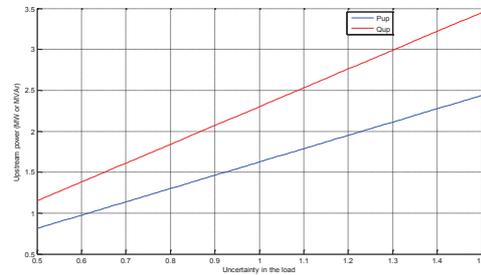
Fig. 13. Upstream power variation in 33-bus system with uncertainty in the variation of loads after installation of two DGs.
