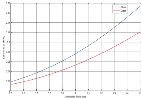
Fig. 15. Losses variations in 33-bus system with uncertainty in the variation of loads after installation of three DGs.
