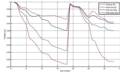
Fig. 4. Bus voltage before and after DGs Installation.
