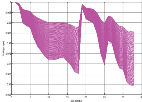
Fig. 14. Bus voltage in 33-bus system with uncertainty in the variation of loads after installation of three DGs.
