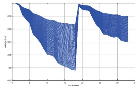
Fig. 8. Bus voltage in 33-bus system with uncertainty in the variation of loads after installation of one DG.
