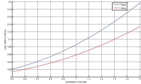
Fig.12. Losses variations in 33-bus system with uncertainty in the variation of loads after installation of two DGs.
