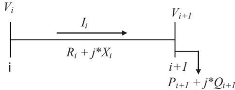
Fig.2. Electrical equivalent of Figure.1.
