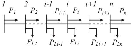
Fig.1. Single-line diagram of a radial distribution network.
