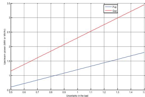
Fig. 16. Upstream power variation in 33-bus system with uncertainty in the variation of loads after installation of three DGs.
