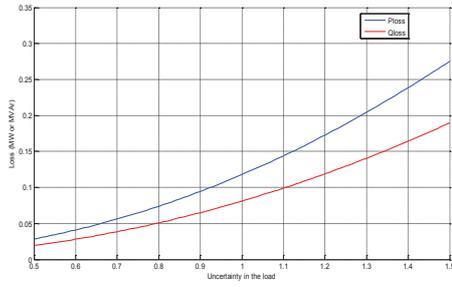
Fig. 9. Losses variations in 33-bus system with uncertainty in the variation of loads after installation of one DG.
