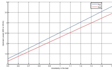
Figure 10. Upstream power variation in 33-bus system with uncertainty in the variation of loads after installation of one DG.
