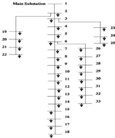
Fig.3.The schematic of a 33-bus radial distribution network.
