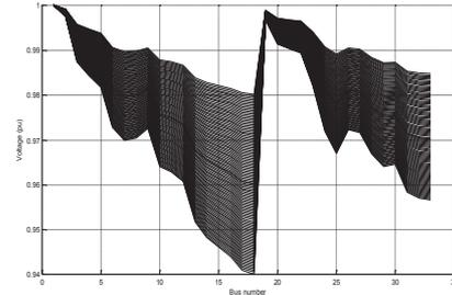
Fig. 11. Bus voltage in 33-bus system with uncertainty in the variation of loads after installation of two DGs.
