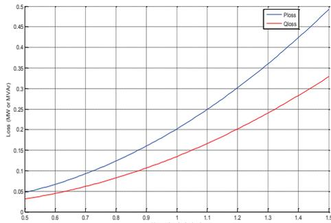
Fig. 6. Losses variations in 33-bus system with uncertainty in the variation of loads without installing DG.
