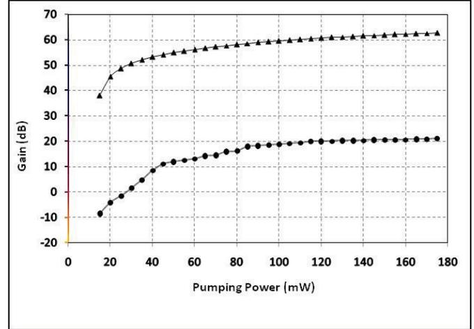
Fig. 5: Experimental results of gain (dB) versus pumping power (mW) for (•) single pass configuration and (▲) double pass dual stage configuration.
