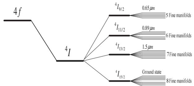
Fig. 2: The energy levels distribution of the erbium atoms
