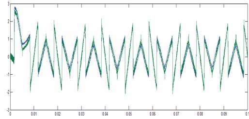
Fig. 4. The injected and the reference currents of filter for the frequency 50 Hz
