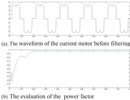
(a). The waveform of the current motor before filtering
