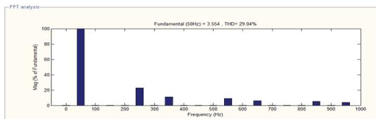
Fig. 8. The harmonic spectrum for the current motor before filtering
