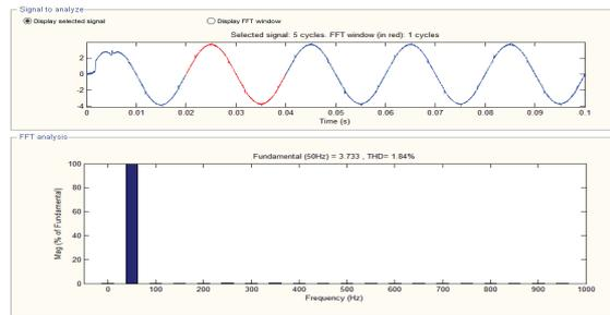
(a). The waveforms of the current motor for 50Hz
