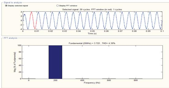
(d). The waveforms of the current motor for 200Hz
