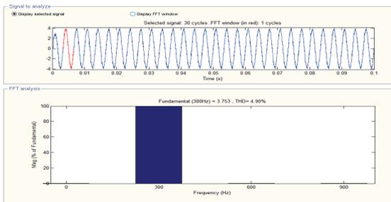
(f). The waveforms of the current motor for 300Hz
