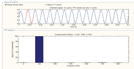
(c). The waveforms of the current motor for 150Hz
