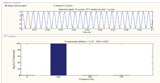
(e). The waveforms of the current motor for 250Hz
