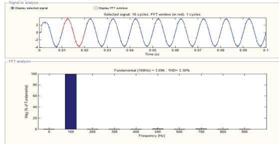
(b). The waveforms of the current motor for 100Hz
