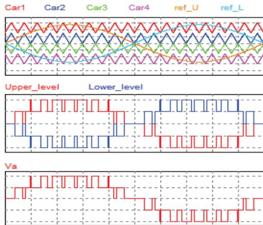
Fig. 11. PODPWM for MMC with even number of sub-modules; N=4
