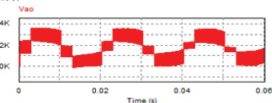
Fig. 17. Leg a output voltage of MMC without balancing algorithm
