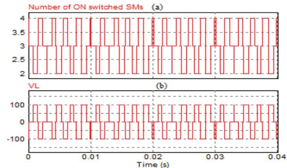
Fig. 8. PDPWM modulation strategy for a 3-SM MMC a) voltage level b) leg *a* upper arm inductor voltage
