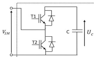
Fig. 2. Topology of a single Sub-Module SM of a MMC converter
