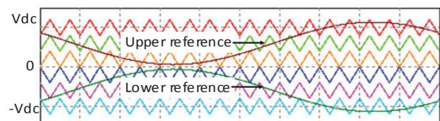
Fig. 13. Proposed PODPWM for a 3-SM MMC converter
