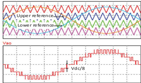
Fig. 7.  $2N+1$  modulation strategy: PDPWM a) carriers disposition b) leg *a* output voltage: 9 levels
