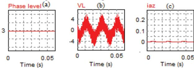
Fig. 15. 3-SM MMC converter leg characteristics a)Number of ON switched SMs b) Inductor voltage c) circulating current
