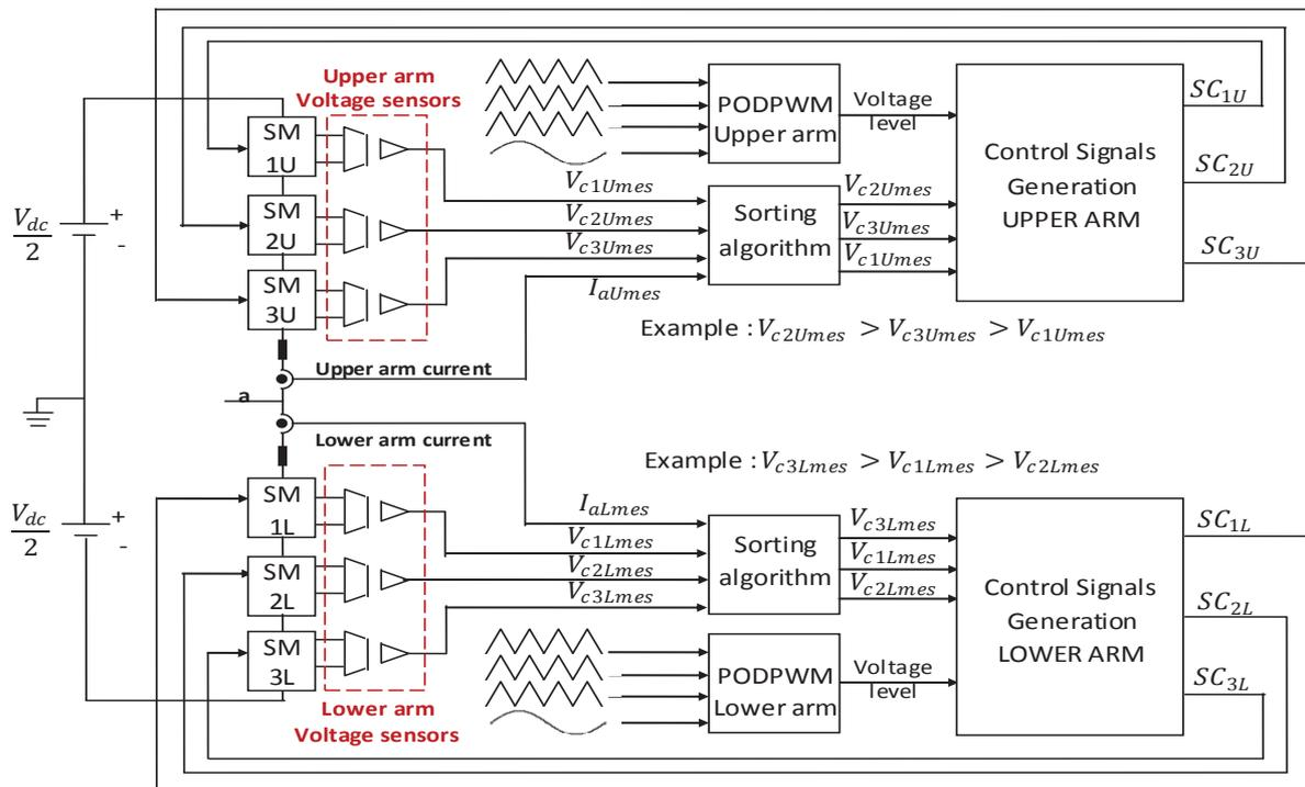
Fig. 19. Block diagram of the proposed algorithm applied for one leg
