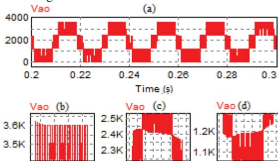
Fig. 20. Three-SM MMC converter output voltage a) output voltage b) zoom on the 3600V level c) zoom on the 2400V level d) zoom on the 1200V level
