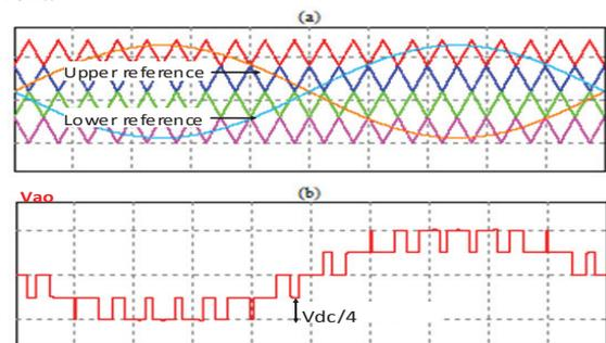
Fig. 3.  $(N+1)$  modulation strategy: APODPWM;  $N=4$  a) carriers disposition b) Simple output voltage: 5 voltage levels
