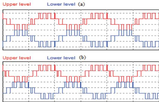
Fig. 14. Upper and lower arms voltage levels a) PODPWM b)PDPWM
