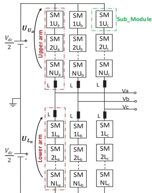
Fig. 1. N-SM Modular Multilevel Converter
