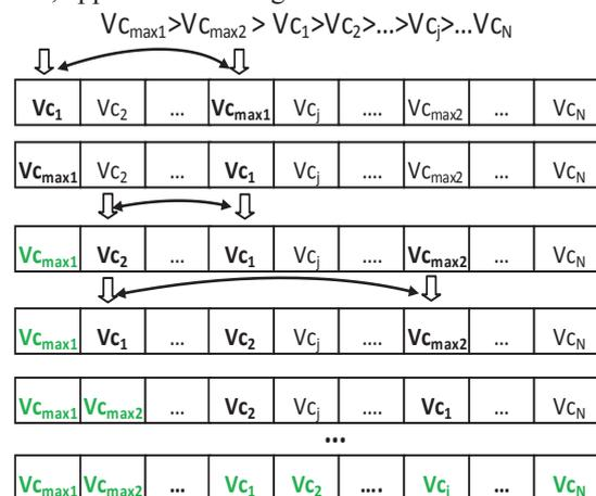
Fig. 18. Sorting algorithm for an N-SM MMC
