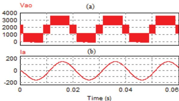
Fig. 16. 3-SM MMC converter a) Simple output voltage b) Line current
