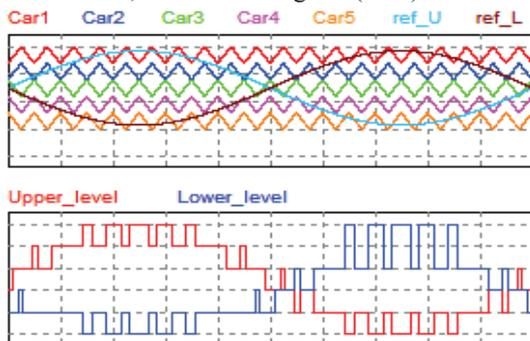
Fig. 12. PODPWM for MMC with odd number of sub-modules; N=5
