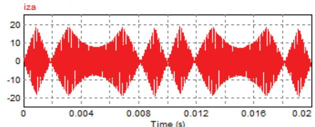
Fig. 10. Leg *a* circulating current under PDPWM modulation strategy
