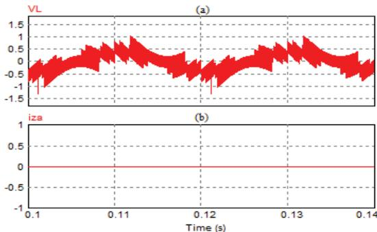
Fig. 6. APODPWM modulation strategy for a 4-SM MMC converter  $V_{dc}=600$  V;  $L=100$   $\mu$ H,  $f_{sw}=10$  kHz a) inductor voltage (2.10-2V/div) b) Leg *a* circulating current  $i_{za}$
