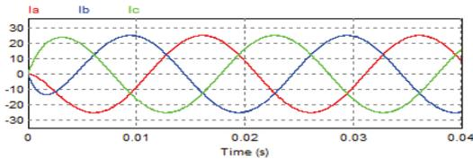
Fig. 4. 3-SM MMC APODPWM modulated converter: line currents (10A/div)
