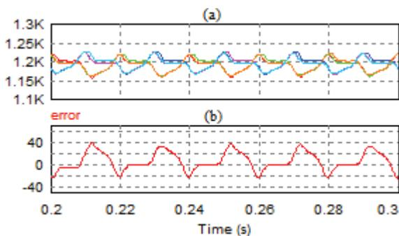
Fig. 21. Voltage balance outputs a) Leg *a* flying capacitors voltages b) error on the capacitor voltage of the first sub module of leg *a* upper arm.
