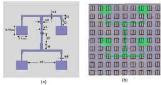
Fig 2. (a) 2 x 2 patch antenna array, dimensions and parameters:  $w_1 = 1.511\text{mm}$ ,  $w_2 = 2.94\text{mm}$ ,  $w_3 = \text{mm}$ ,  $w_4 = 0.516\text{mm}$ ,  $w_5 = 17.02\text{mm}$ ,  $l_1 = 2.511\text{mm}$ ,  $l_2 = 7.5\text{mm}$ ,  $l_3 = 10\text{mm}$ ,  $l_4 = 7.5\text{mm}$  (b) 2 x 2 patch antenna array with superstrate
