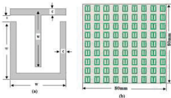
Fig 1. Configuration of U and T shaped metamaterial superstrate (a) The unit cell dimensions and parameters  $w = 5\text{mm}$ ,  $c = 0.66\text{mm}$  (b) 9x9 array of the U and T shaped metamaterial.
