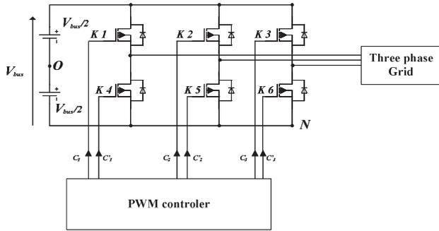
Fig. 5 Three phase voltage inverter connected to a grid.
