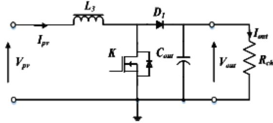
Fig. 3. Typical structure of DC-DC boost converter.
