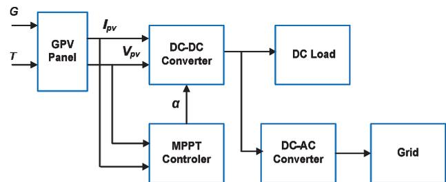
Fig. 1. Blocks of photovoltaic conversion chain.
