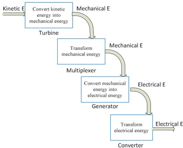
Fig. 6 Blocks of wind conversion chain.
