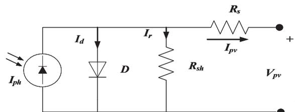
Fig. 2. Equivalent electric diagram of a PV cell [1].
