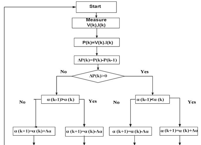
Fig. 4. Flow chart of perturbation and observation algorithm.
