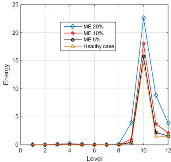
Fig. 7. Energy calculation from stator current for healthy and faulty cases
