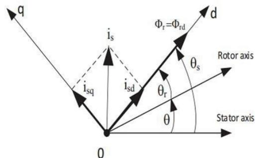
Fig. 2. Stator current space vector and its component
