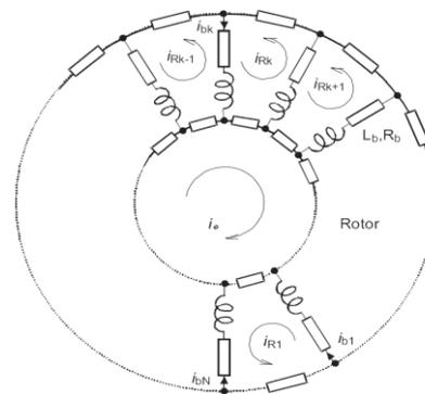
Fig.1. Equivalent Rotor mesh circuit
