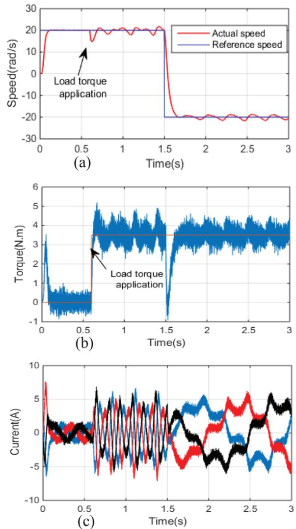
Fig. 4. Faulty motor with mixed eccentricity fault ( $ME 10\%$ ): (a) Rotor speed, (b) Stator current, (c) Electromagnetic torque.
