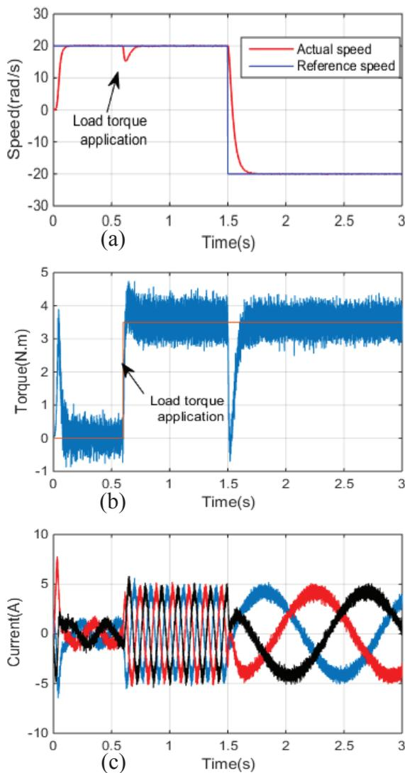
Fig. 3. Healthy condition of the motor: (a) Rotor speed, (b) Stator currents, (c) Electromagnetic torque.
