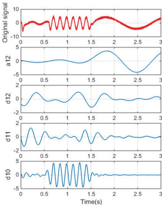
Fig. 5. DWT analysis of current for the healthy machine
