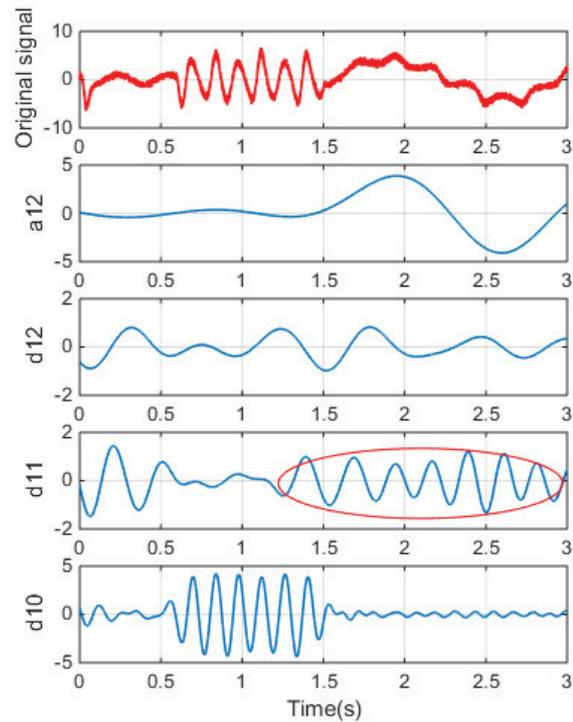
Fig. 6. DWT analysis of current for faulty machine under (ME 10%)
