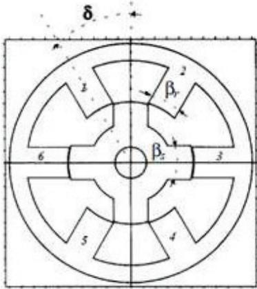
Fig. 2 . The angle  $\delta$  corresponding to displacement of a phase in relation to another
