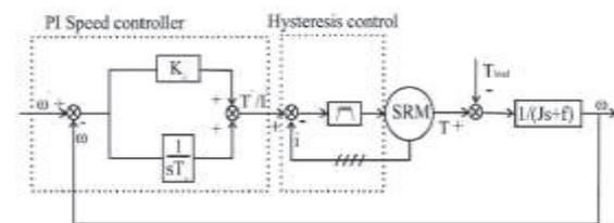
Fig.6. Closed-loop speed and current control block diagram of a SRM.
