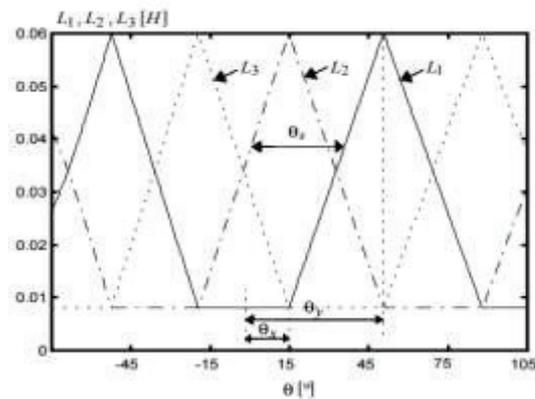
Fig. 1. SRM linear model. Inductance profile of each phase.
