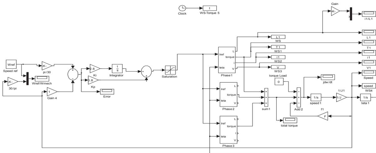
Fig. 3. Matlab/Simulink diagram of SRM linear model
