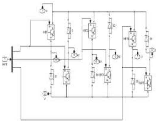
Fig. 5. H-bridge asymmetric converter
