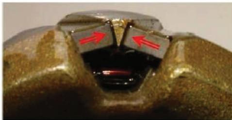
Fig. 2. Rotor of HE2A with magnets inserted between claws
