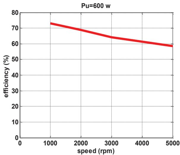
Fig. 9. HE2A efficiency versus speed.
