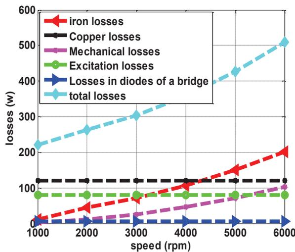
Fig. 6. Calculated alternator losses at 600W.
