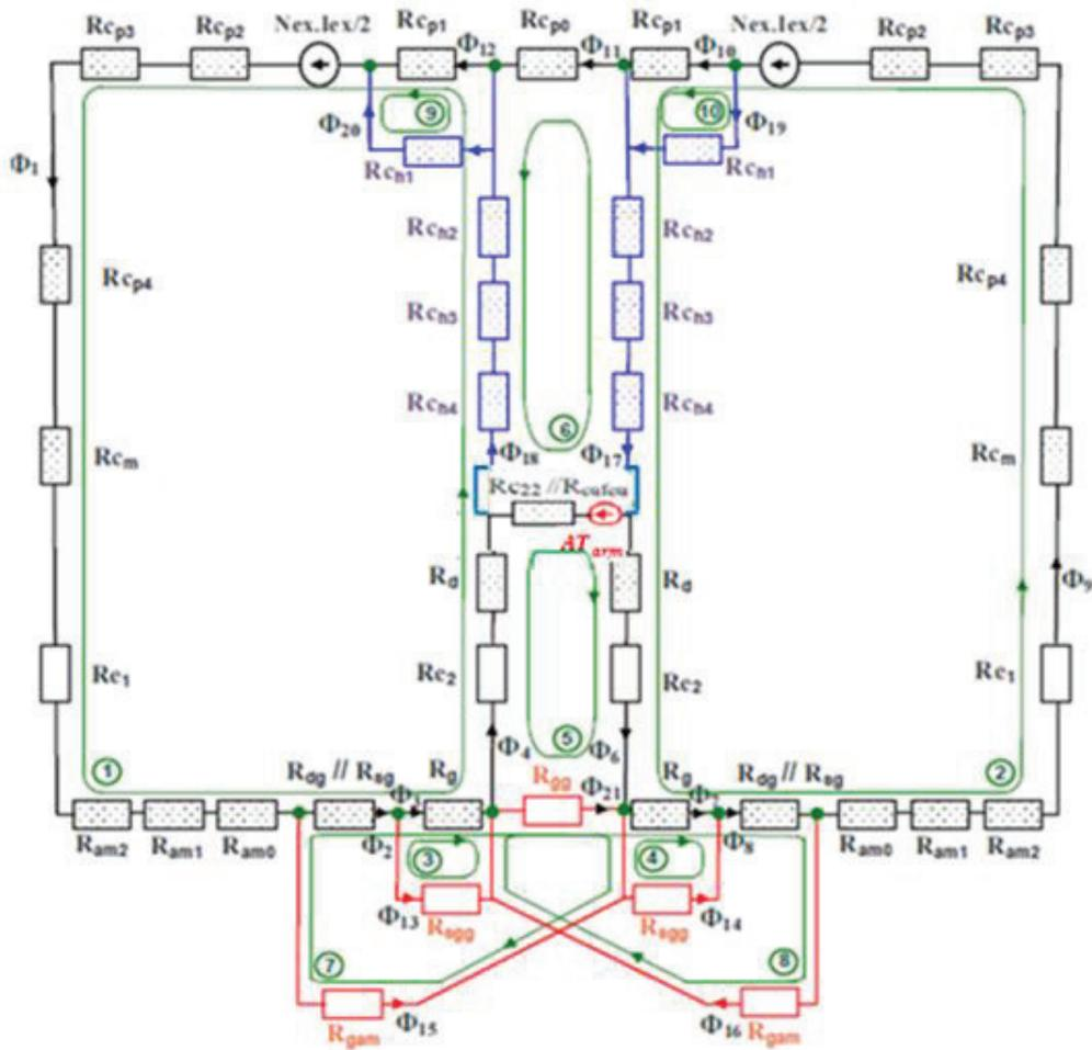
Fig. 4. HE2A reluctance network within the d-axis accounting for the armature magnetic reaction and the saturation.
