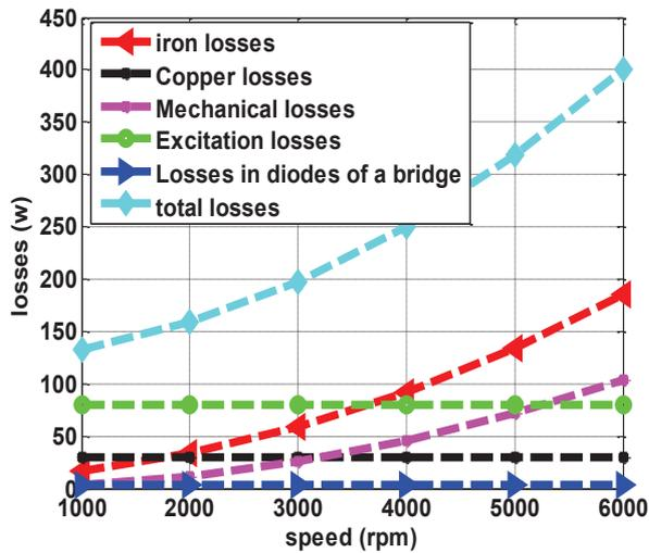
Fig. 5. Calculated alternator losses at 300W.
