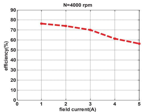
Fig. 8. HE2A efficiency versus field current
