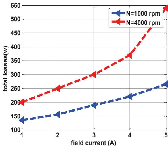
Fig. 7. Calculated load total losses versus field current.
