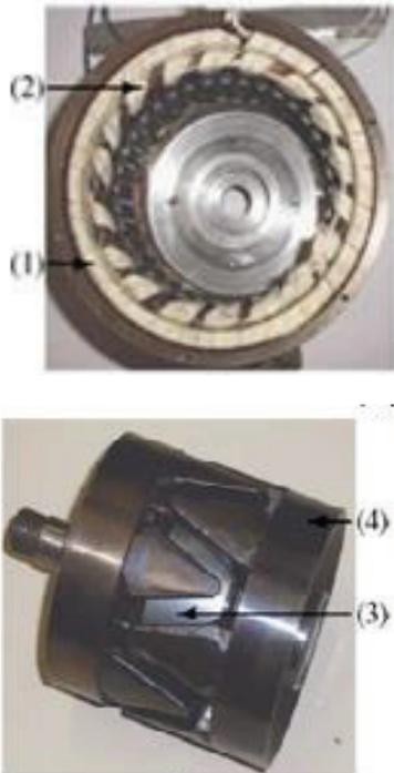
Fig. 1. Built prototype of the SE2A. Legend: (a) Sator of the SE2A, (b) rotor of the SE2A, (1) half of the sator DC-excitation ring winding, (2) armature en winding, (3) non-magnetic core, (4) magnetic collector.
