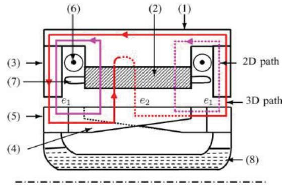
Fig. 3. Flux paths through the magnetic circuit of the HE2A. Legend: (1) to (5) same as in Fig. 1, (6): half of the sator DC-excitation winding, (7): armature end-winding, (8): non-magnetic core holding the two magnetic rings.
