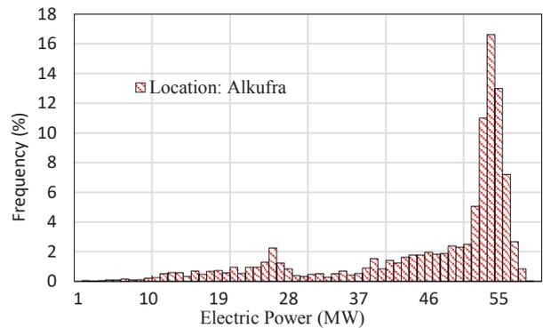
Fig. 7. Power histogram (Frequency distribution) of CSP power plant using PTC without storage at Alkufra area with an optimum solar multiple of 1.3.
