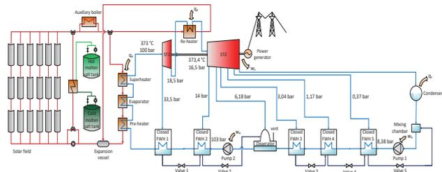
Fig. 6. Reheat regenerative Rankine cycle based on the commercial PTC CSP plants, typical configuration, [12]
