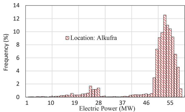
Fig. 8. Power histogram (Frequency distribution) of CSP power plant using PTC with storage at Alkufra area with an optimum solar multiple of 2.
