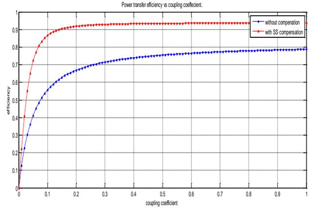
Fig. 2. Transfer power efficiency as a function of coupling coefficient with and without SS compensation
