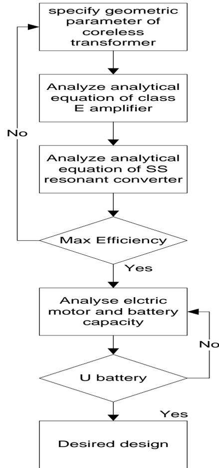
Fig.8 Iterative process applied to design proposed WBC system
