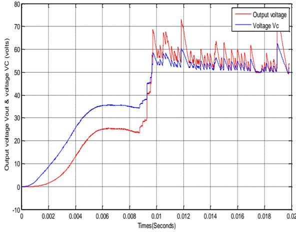
Fig.10 voltage across C3 capacitor and output voltage of the proposed WBC system
