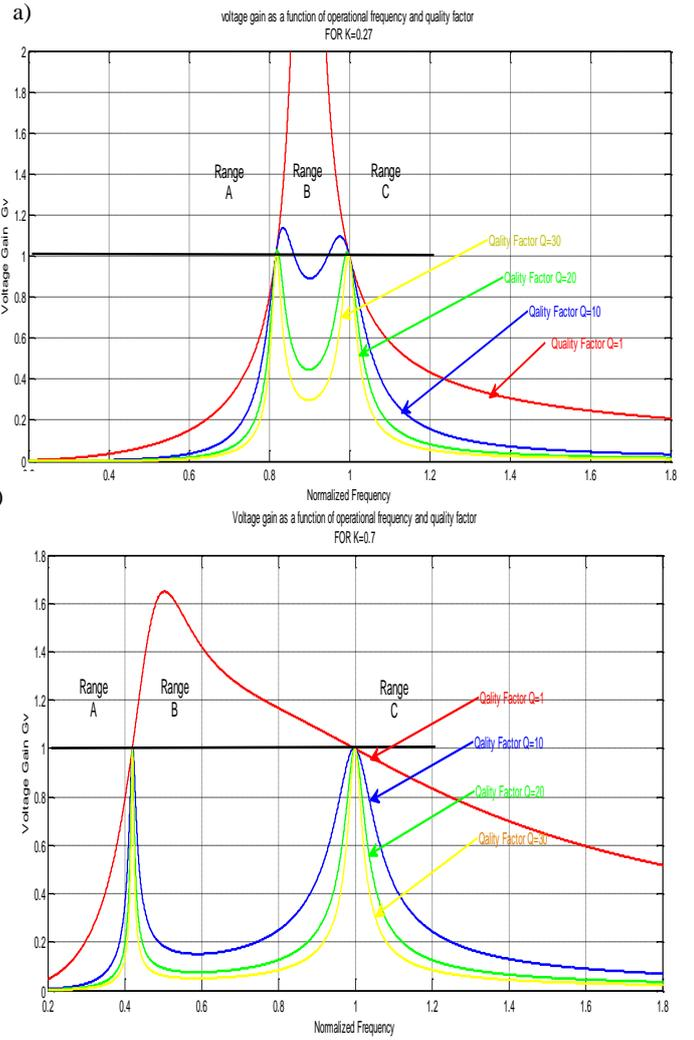
Fig. 4. Voltage gain as function of normalized frequency and quality factor for a)  $K=0.2$ . b)  $K=0.7$
