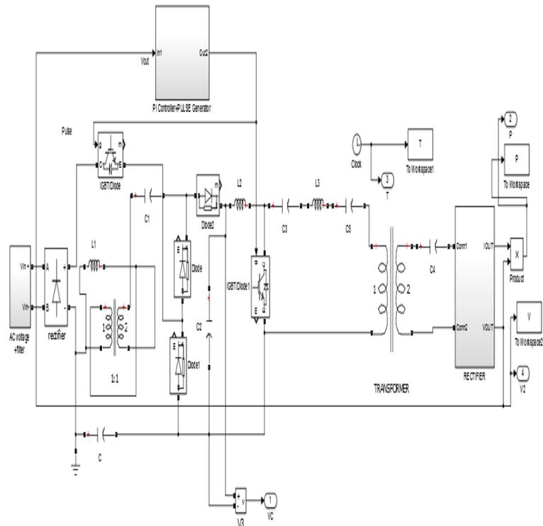
Fig.7 Matlab/simulink bloc diagram of the proposed WBC system
