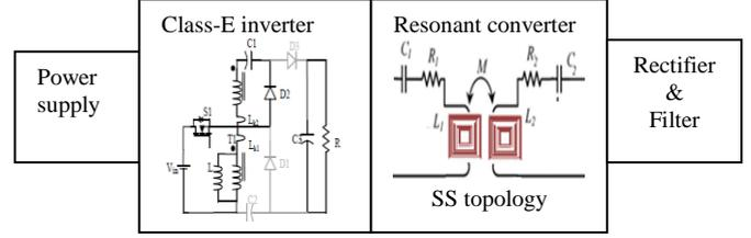
Fig.1 Bloc diagram of the proposed wireless charger battery system
