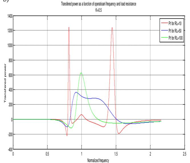
Fig. 3. Transferred power as a function of normalized frequency and load resistance  $R_L$ , for a)  $K=0.27$  .b)  $K=0.5$
